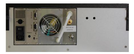
**Hydrogen Outlet**: Hydrogen pressure is available at the OUTLET  $H_2$  output on the back of the instrument. This outlet is equipped with a stainless steel Swagelok 1/8" fitting.
