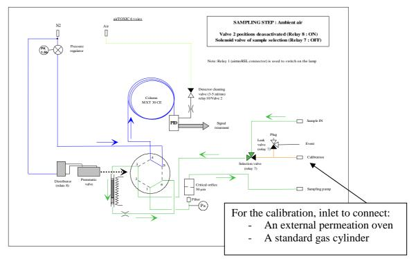
With option internal calibration, the pneumatic scheme is:
