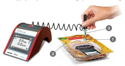
2. Place a septum 1 on the product/package 2 to be measured/analysed. This ensures leak-free gas extraction and thus accurate measuring.
