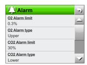
**O2 Alarm limit** Set the appropriate value for the  $O_2$  concentration (0.1 - 100%).
