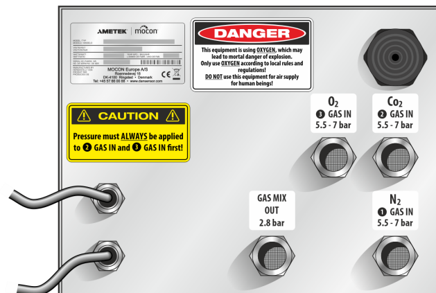
Abb. 3. Dansensor® MAP Mix 9001 ME Anschlüsse
