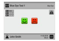
Thus, if you press the 🙂 button, the test result will subsequently be indicated and registered as **OK**, whereas pressing the 🗮 button will indicate and register the result as **Error**.
