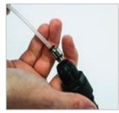
Screw the quick-connect fitting back into the filter holder and hand-tighten.
