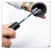
Using a 13mm soocket, unscrew the bronze dust filter and remove it from its position inside the rubber housing
