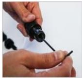
Use the 3mm allen wrench to provide a final tighten.
