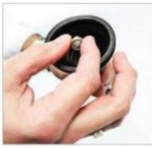
Discard the old filter and replace it with a new filter
