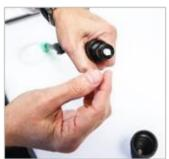
Once the rubber housing has been removed, remove and discard the cellulose filter from the holder found at the end of the wand
