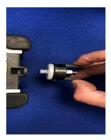
Change the filter and reassemble by turning it clockwise.
