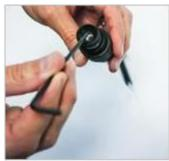
Using a 3mm Allen wrench, release the nut inside the filter holder.
