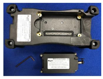
The picture shows the battery removed from the instrument
