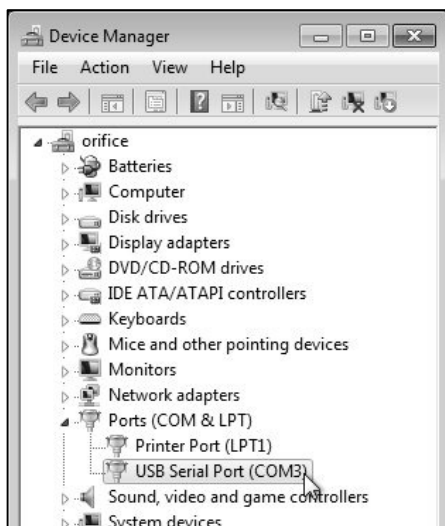
Fig. 3: Example: entry of the virtual COM port (in this example COM3) in the Windows Device Manager of a PC named 'orifice'.
