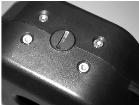
Fig. 11: Internal calibration switch in 'measurement' position.
