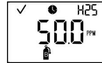
Bump test apply gas
