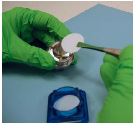
Fig.11.6 Placing a new filter-paper in the unit
