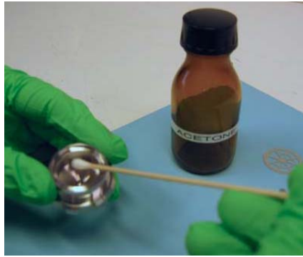
Fig.11.5 Cleaning the surfaces of the internal air-filtration unit
