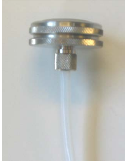
Fig.2.9 Fitting the external filter UD5023 to sampling tube
