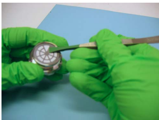
Fig.11.4 Removing the retaining disc and old filter-paper
