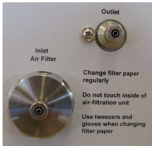
Fig.11.1 The internal air-filtration unit mounted on the back panel of the monitor.
