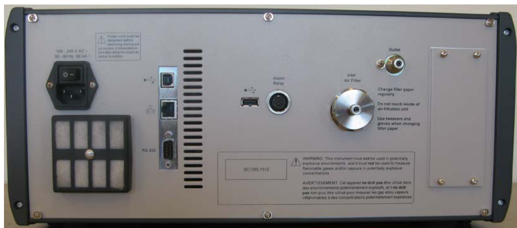
Fig.11.9 Back panel of the 1512 showing the ventilation unit
