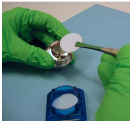
Fig.11.6 Placing a new filter-paper in the unit
