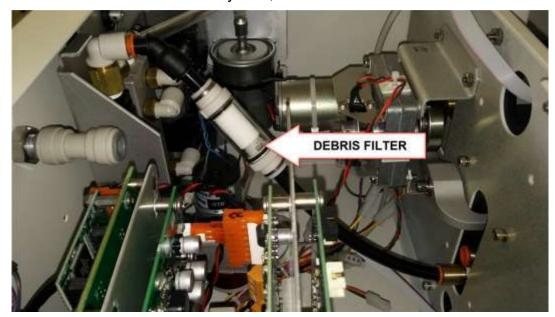
Figure 6-3 Debris Filter Location
