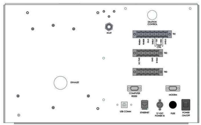
Figure 2-5 BC 1054 Rear Panel Connections
