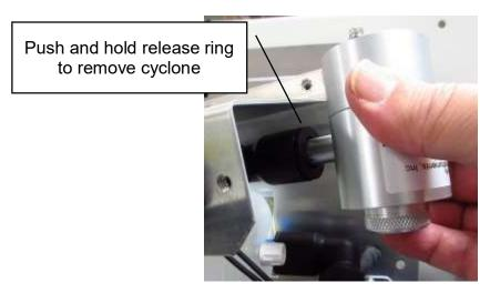
Figure 6-9 Push and hold release ring
