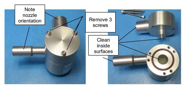
Figure 6-10 Note nozzle orientation of dilution system cyclone. Remove screws and clean interior surfaces for full cyclone cleaning.
