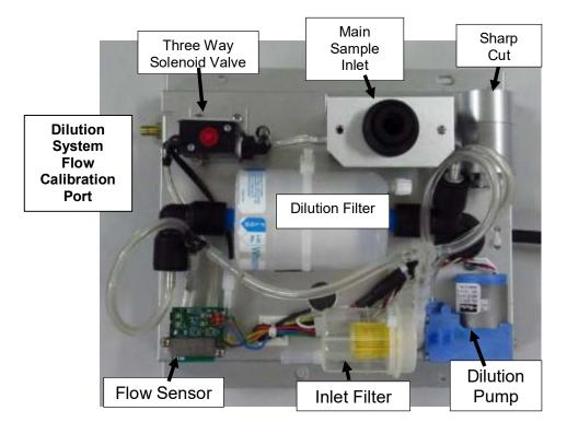
Figure 4-3 Major Components of the Dilution Flow System
