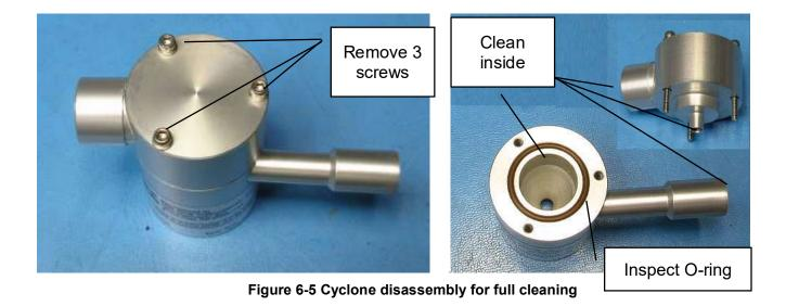
Full cleaning of the cyclone requires accessing the conical chamber inside. All of the inside surfaces must be cleaned. Isopropyl alcohol and cotton-tipped applicators work well.
