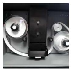
Figure 5-9 Loosening the Tape for Cover Removal
