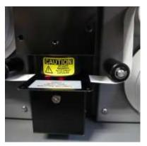
Figure 5-14 Inserting the Neutral Density Span Membrane
