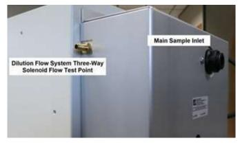
Figure 5-5 Dilution Flow System Air Flow Locations
