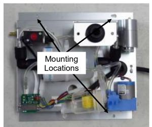
Figure 2-8 Dilution Flow System Mounting Screw Locations
