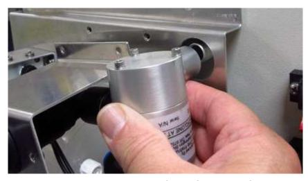
Figure 6-8 Pull cyclone away from BC 1054 inlet fitting
