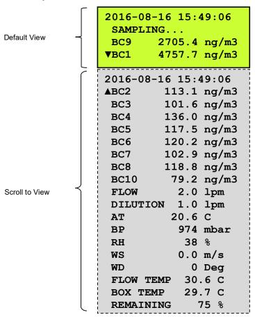
Figure 3-2 Main Sampling Screen Format
