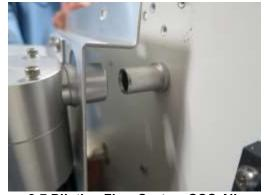
Figure 2-7 Dilution Flow System SCC Alignment
