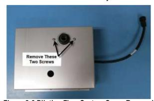
Figure 2-6 Dilution Flow System Cover Removal
