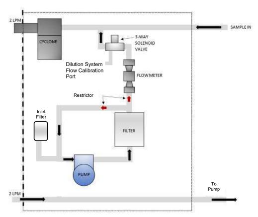
Figure 4-2 BC 1054 Dilution Flow System Diagram
