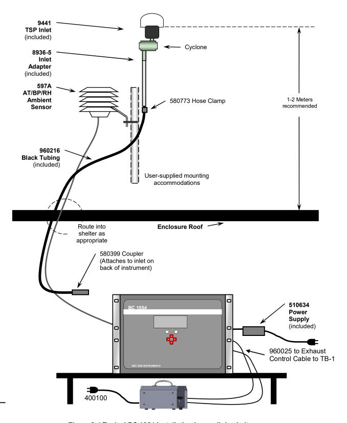
Figure 2-4 Typical BC 1054 Installation in a walk-in shelter
