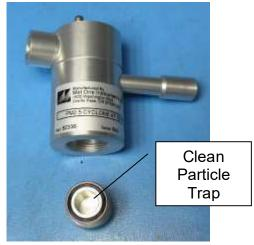
Figure 6-4 Unscrew and clean particle trap
