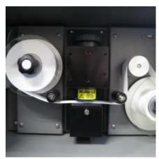
Figure 5-10 Removing the Measurement Head Cover
