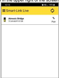
3. On initial setup, your GAS•TRAC LZ-30 will be shown as "Atmosic Bridge", because no serial number has been assigned to it yet. Below that will be a list of letters and numbers separated by colons, which is the Bluetooth ID. If you have multiple LZ-30s, you may need to use the ID to know which instrument to connect to. To do so, press and release the ON/MENU button twice on the LZ-30. The Bluetooth ID for that instrument will be shown.
