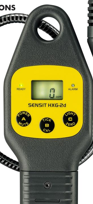
7. Extend the goose neck (the PPM/LEL sensor and cap is at the tip).
