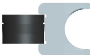
Figure 4-20: Replace Mesh in Filter Holder
