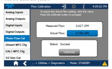
Figure 5-9. Photometer Flow Calibration Screen
