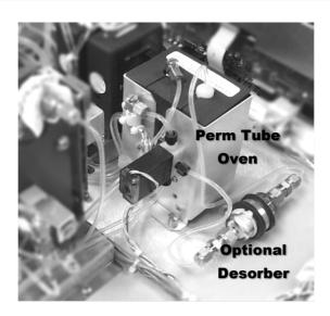
Figure 2-28. Permeation Tube Gas Generator Option
