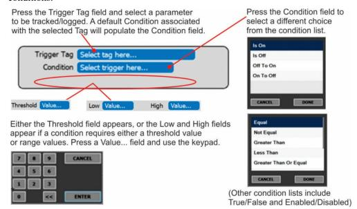
Figure 2-49. Datalog - Conditional Trigger Configuration
