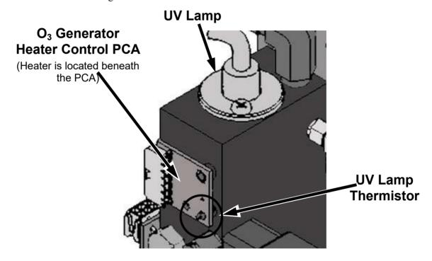
Figure 8-16. O<sub>3</sub> Generator Temperature Thermistor and DC Heater Locations
