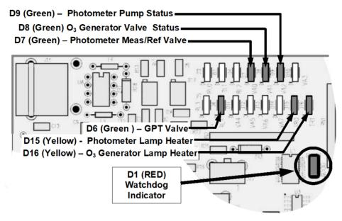
Figure 7-2. Relay PCA Status LEDS Used for Troubleshooting
