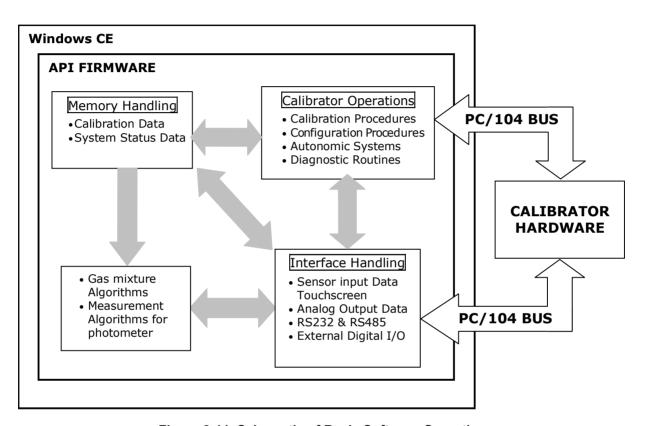
Figure 8-11. Schematic of Basic Software Operation
