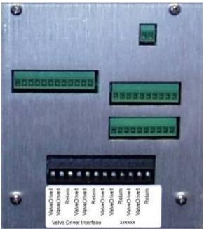
Figure 2-11. Valve-Driver Interface
