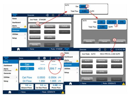
Figure 5-5. O<sub>3</sub> Photometer Performance Verification
