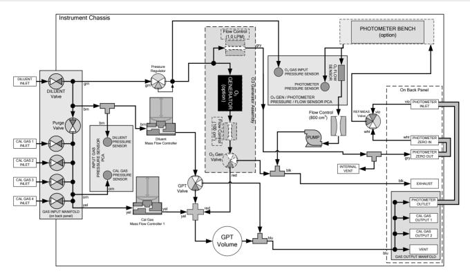
Figure 2-25. Internal Pneumatics for Calibrator with Optional O<sub>3</sub> Generator and Photometer
