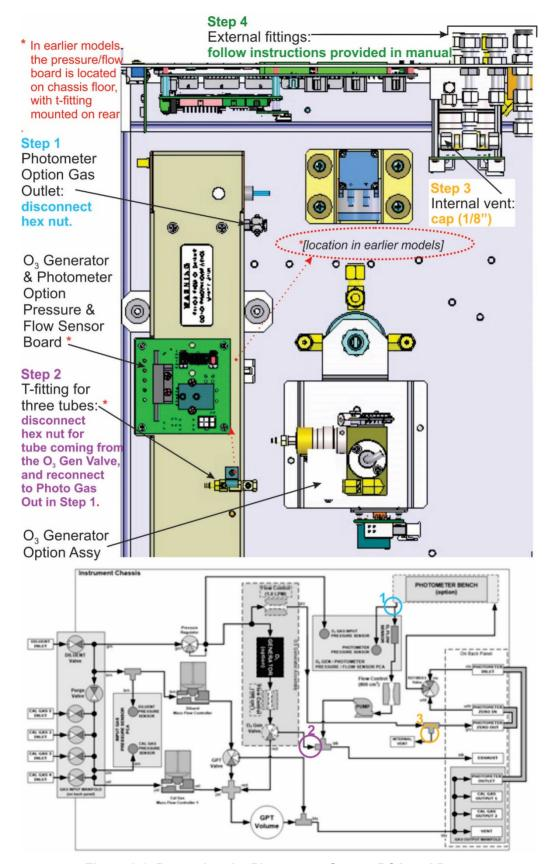
Figure 6-6. Bypassing the Photometer Sensor PCA and Pump
