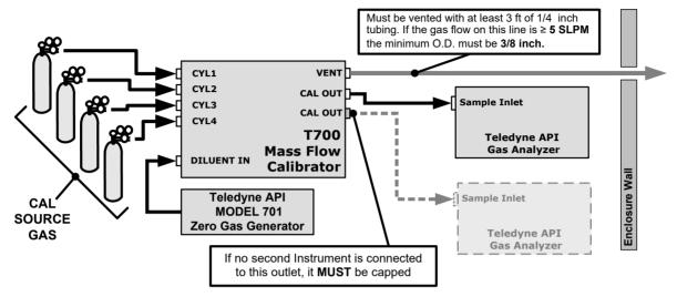
Figure 2-19. Setup - Connecting the Basic Calibrator to a Sample Manifold
