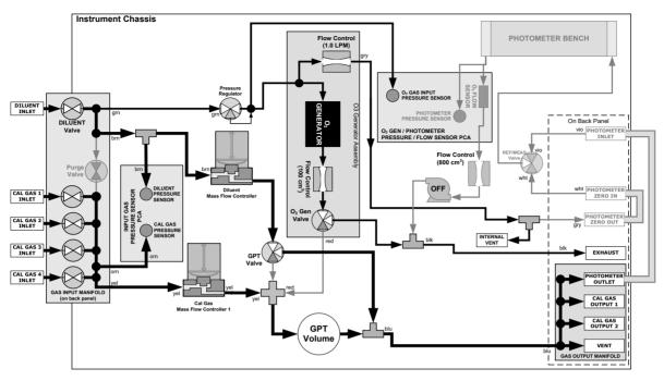
Figure 3-3. Gas Flow with O<sub>3</sub> Options when Generating Non-O<sub>3</sub> Source Gas
