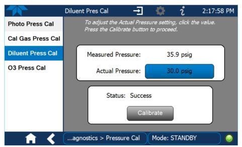
Figure 5-13. Pressure Sensor Calibration Page (Diluent Example)
