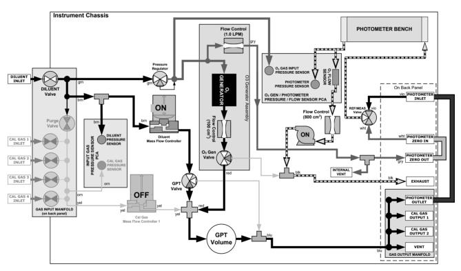
Figure 3-11. Gas Flow with O<sub>3</sub> Options during GPTPS Mode
