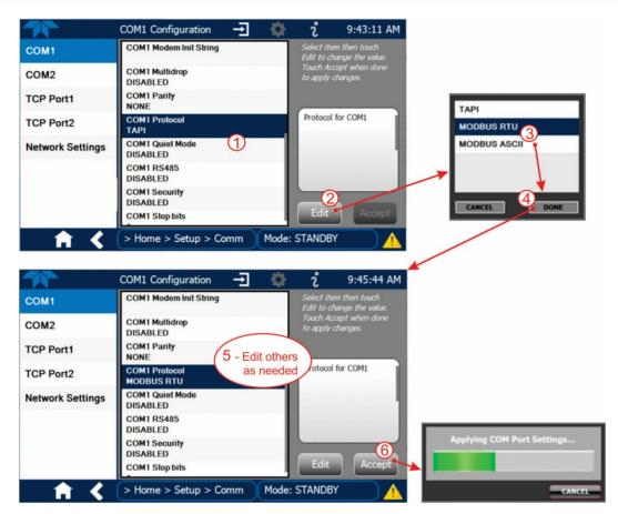
Figure 4-2. MODBUS via Serial Communication (example)
