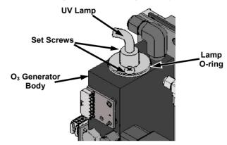
Figure 6-11. O<sub>3</sub> Generator UV Lamp Location
