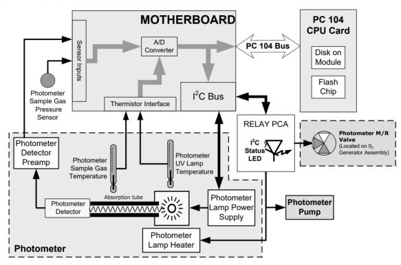
Figure 8-21. O<sub>3</sub> Photometer Electronic Block Diagram
