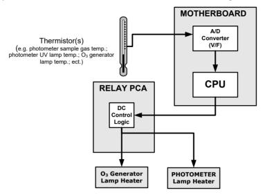
Figure 8-6. Heater Control Loop Block Diagram.
