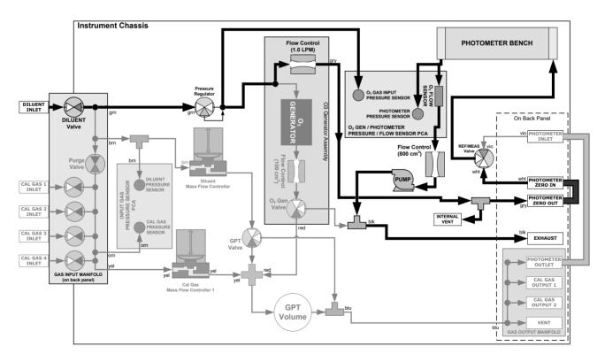
Figure 8-18. O<sub>3</sub> Photometer Gas Flow - Reference Cycle
