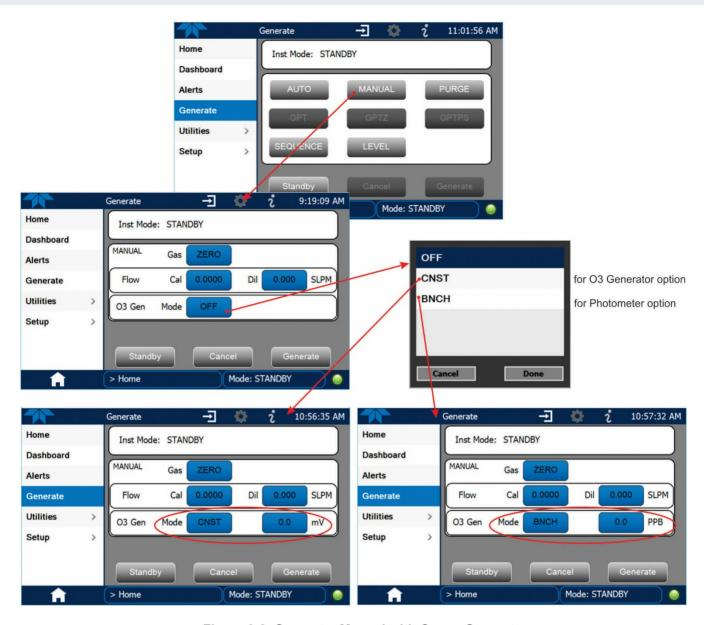
Figure 3-8. Generate>Manual with Ozone Generator
