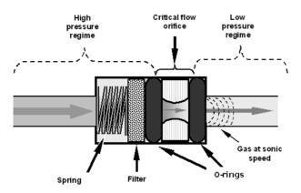
Figure 8-2. Flow Control Assembly & Critical Flow Orifice
