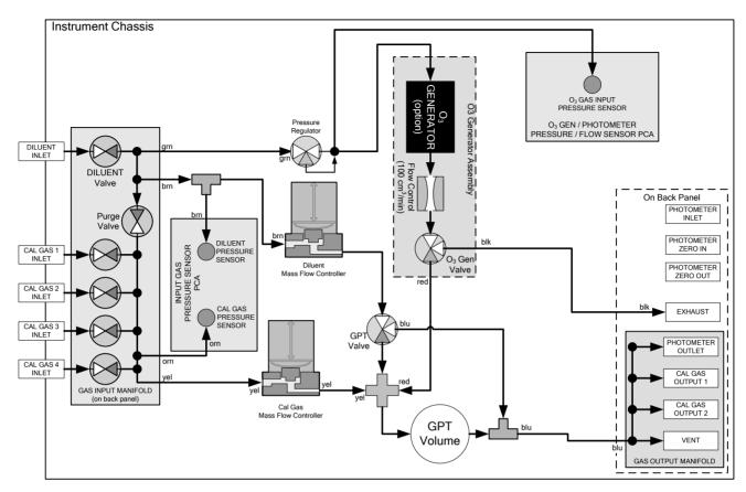
Figure 2-24. Internal Pneumatics for Calibrator with Optional O<sub>3</sub> Generator and GPT Chamber
