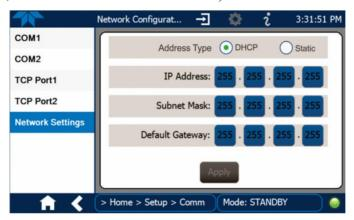
Figure 2-64. Communications Configuration, Network Settings
