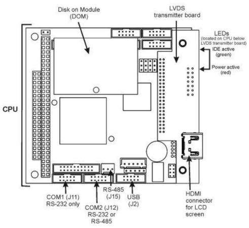
Figure 8-4. Calibrator CPU Board Annotated
