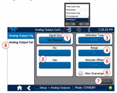
Figure 2-62. Analog Output Configuration
