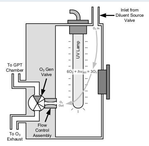
Figure 8-12. O<sub>3</sub> Generator Internal Pneumatics
