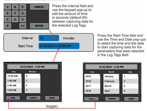
Figure 2-48. Datalog Periodic Trigger Configuration
