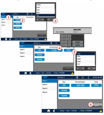
Figure 2-37. Calibration Gas Inlet Ports Setup
