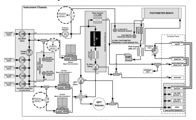
Figure 5-12. Pressure Monitor Points with O<sub>3</sub> Options and Multiple Cal MFCs Installed
