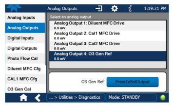
Figure 7-5. Analog Outputs Page Example
