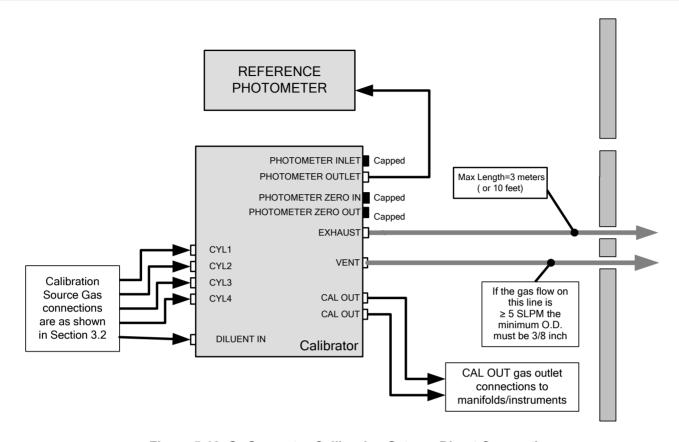
Figure 5-10. O<sub>3</sub> Generator Calibration Setup - Direct Connections
