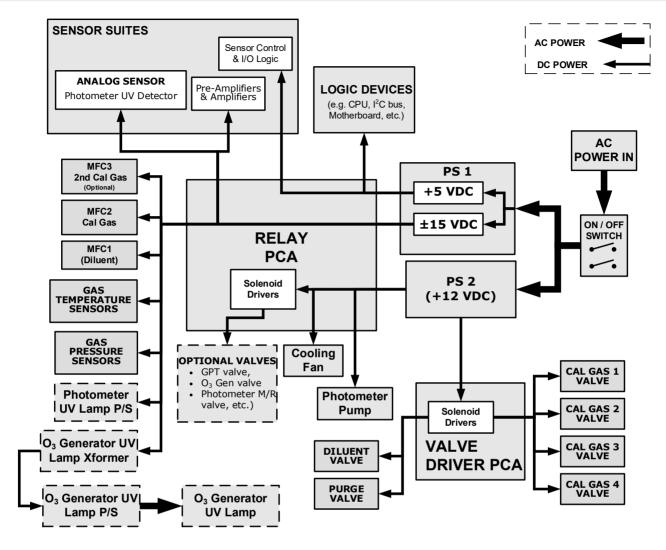
Figure 8-9. Power Distribution Block Diagram
