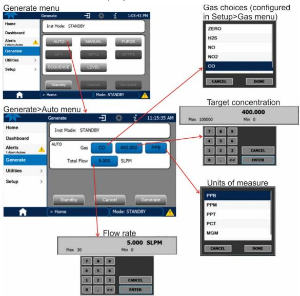
Figure 3-6. Auto Generate Calibration Mixtures
