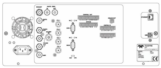
Figure 2-2. Calibrator Rear Panel Layout
