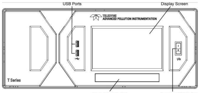
Model Name Label Figure 2-1. Calibrator Front Panel Layout
