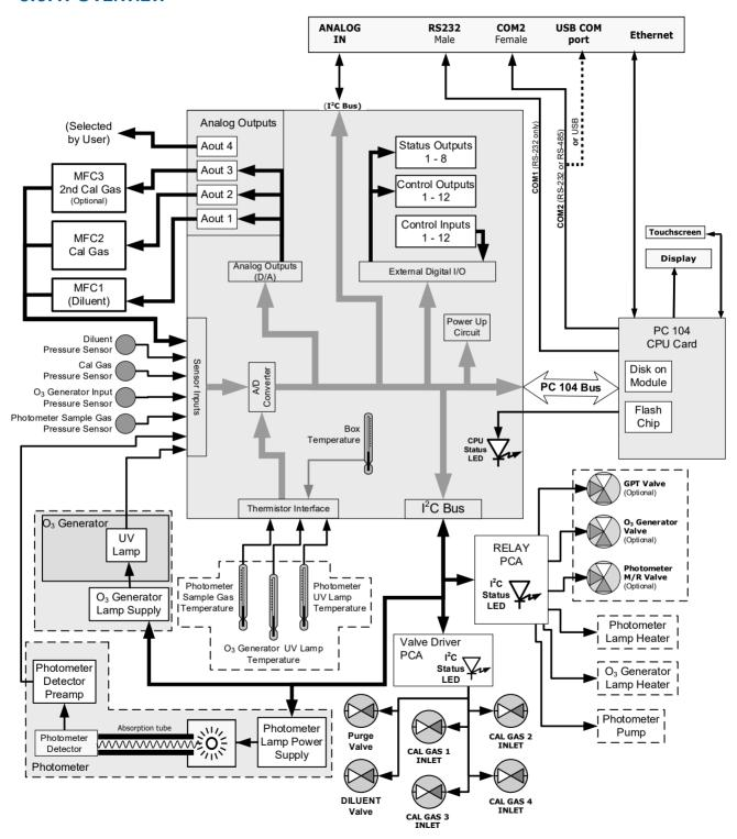
Figure 8-3. Electronic Block Diagram
