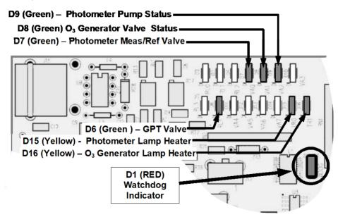
Figure 8-7. Status LED Locations - Relay PCA
