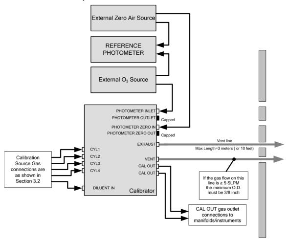
Figure 5-6. External Photometer Validation Setup - Direct Connections
