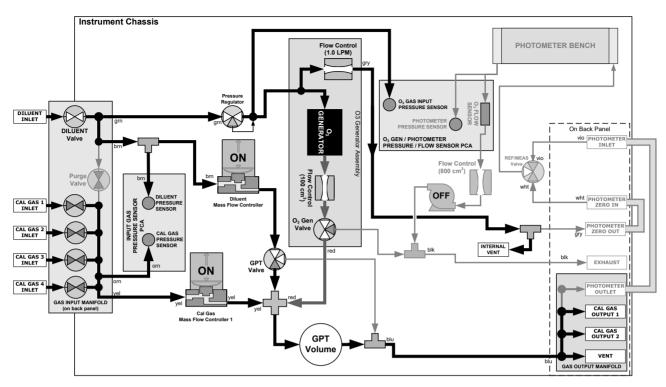
Figure 3-12. Gas Flow with O<sub>3</sub> Options during GPT Mode
