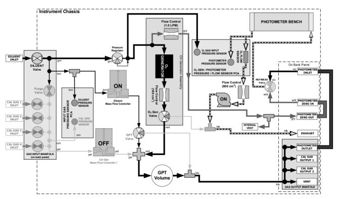
Figure 3-4. Gas Flow with  $O_3$  Options when Generating  $O_3$
