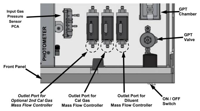
Figure 5-2. Location of MFC Outlet Ports
