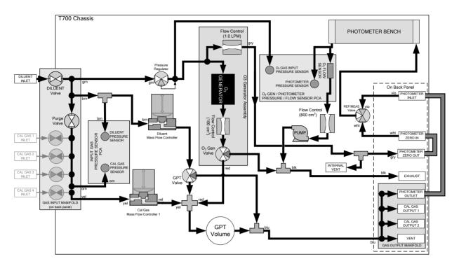
Figure 3-9. Gas Flow with O<sub>3</sub> Options during Purge mode
