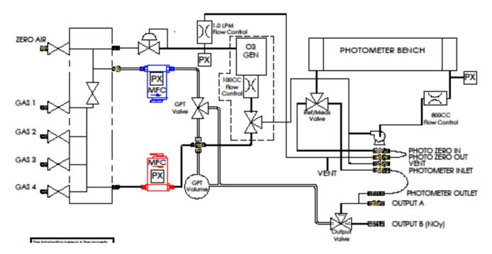
Figure 2-31. Internal Pneumatics with Optional Dual Gas Output (NO<sub>y</sub> – Special)
