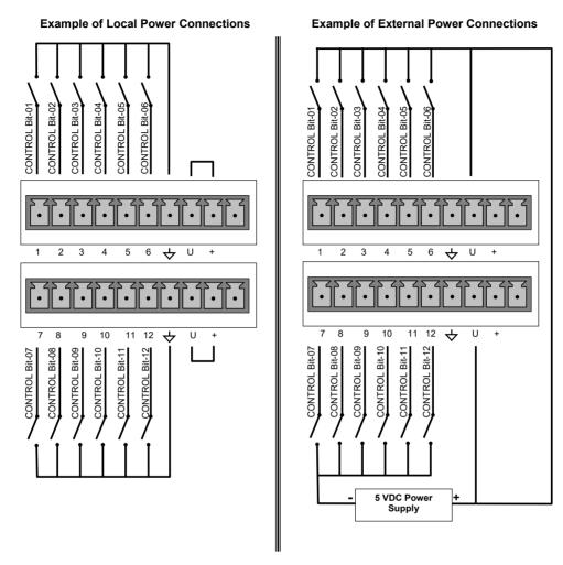
Figure 2-7. Calibrator Digital Control Input Connectors
