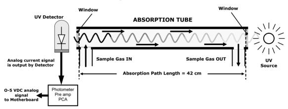
Figure 8-19. O<sub>3</sub> Photometer Absorption Path
