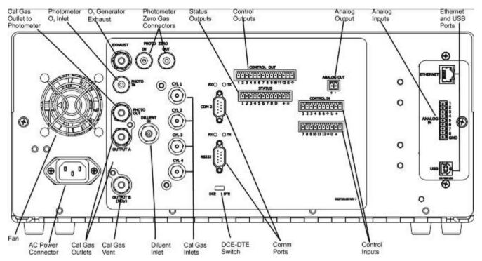
Figure 2-30. Rear Panel with Dual Output Option
