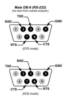
Figure 2-15. Rear Panel Connector Pin-Outs for RS-232 Mode
