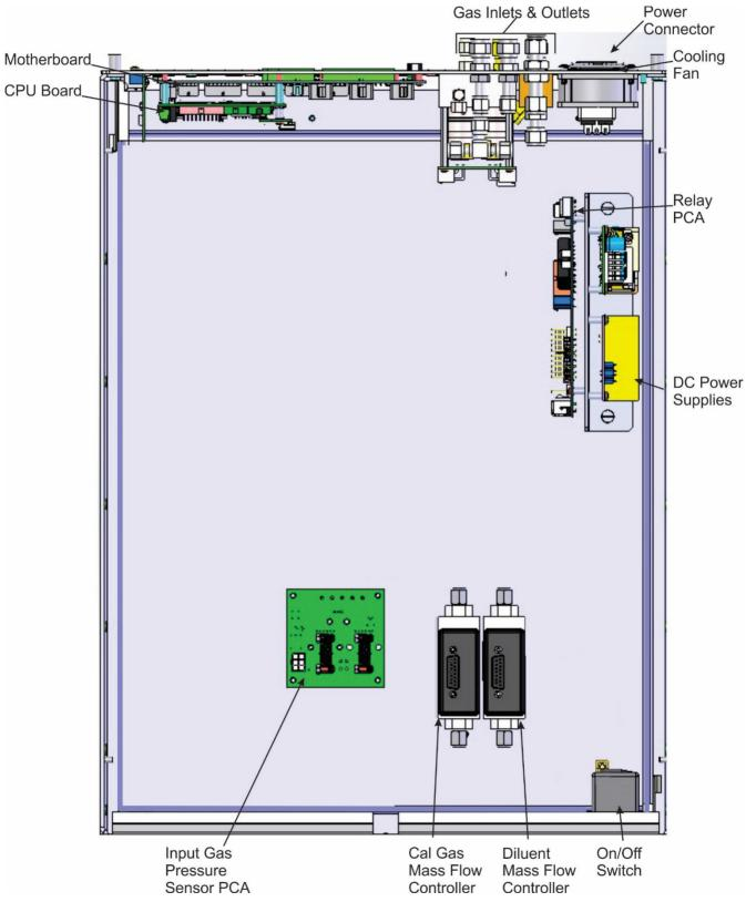
Figure 2-3. Calibrator Internal Layout - Top View - Base Unit
