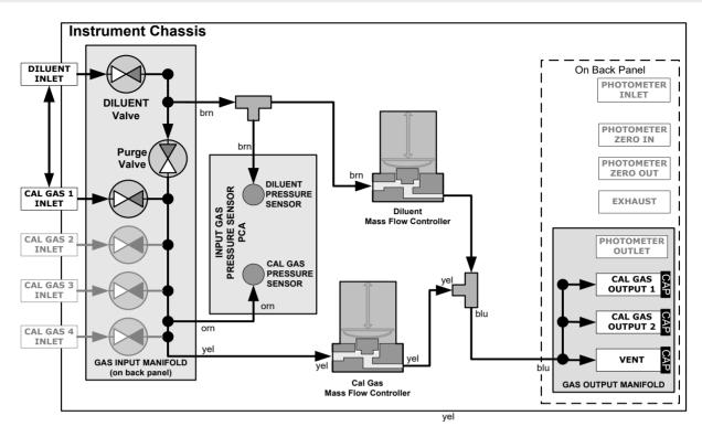
Figure 6-8. Gas Flow for Auto-Leak Check of Base Model Calibrators
