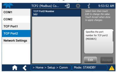
Figure 4-1. MODBUS via Ethernet
