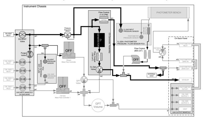
Figure 3-1. Gas Flow with O<sub>3</sub> Generator and Photometer Options during Standby Mode
