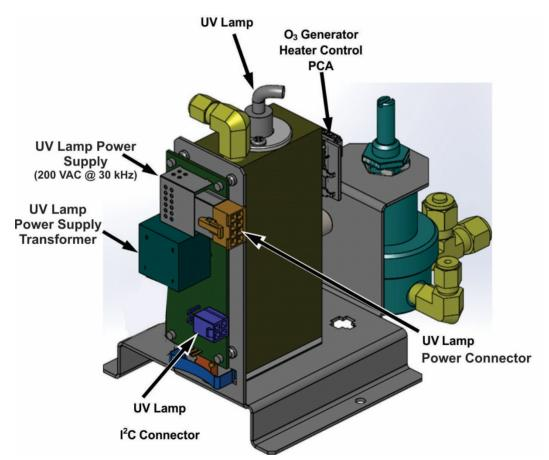
Figure 8-15. O<sub>3</sub> Generator Electronic Components Location
