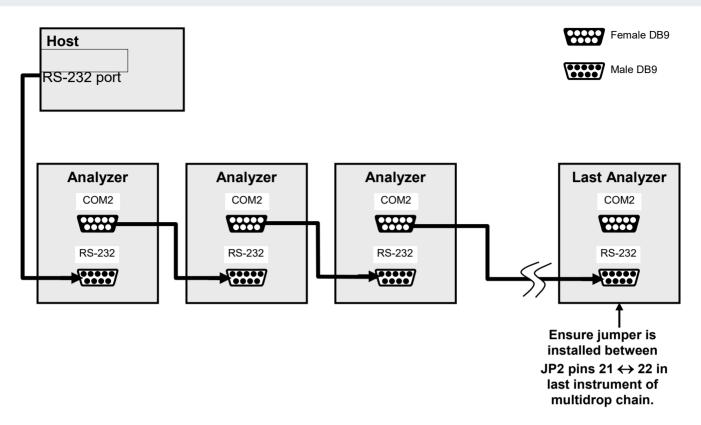
Figure 2-18. RS-232-Multidrop PCA Host/Analyzer Interconnect Diagram
