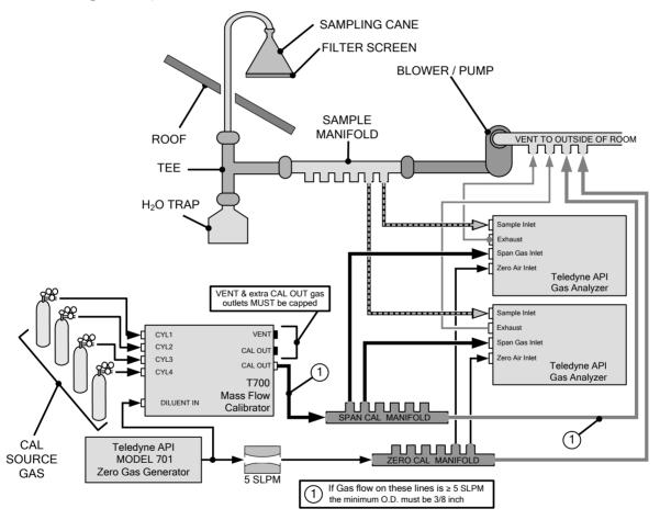
Figure 2-22. Setup - Connecting the Calibrator to a Dual Span Gas / Zero Air Manifold
