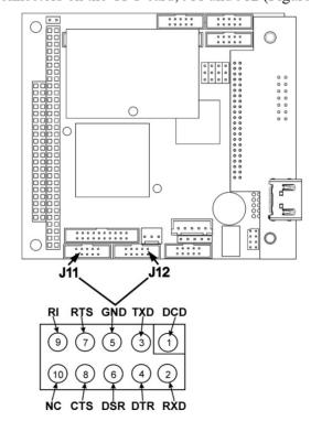
Figure 2-16. Default Pin Assignments for CPU COMM Port Connector (RS-232).
