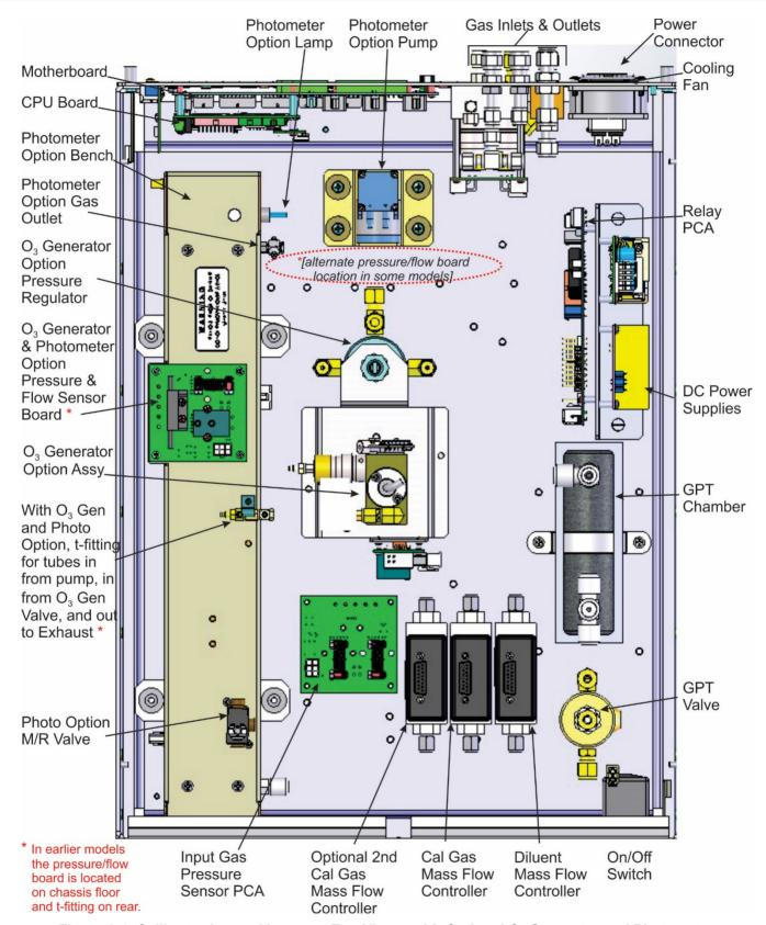
Figure 2-4. Calibrator Internal Layout - Top View - with Optional O<sub>3</sub> Generator and Photometer
