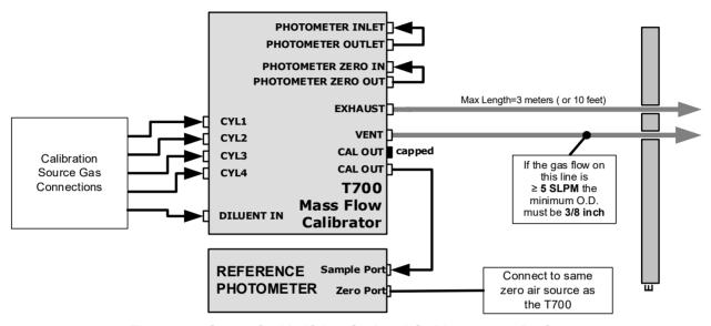
Figure 5-4. Set up for Verifying Optional O<sub>3</sub> Photometer Performance
