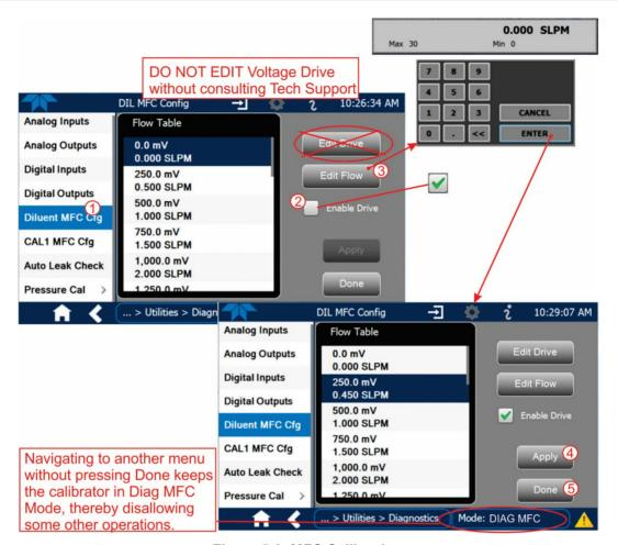
Figure 5-3. MFC Calibration
