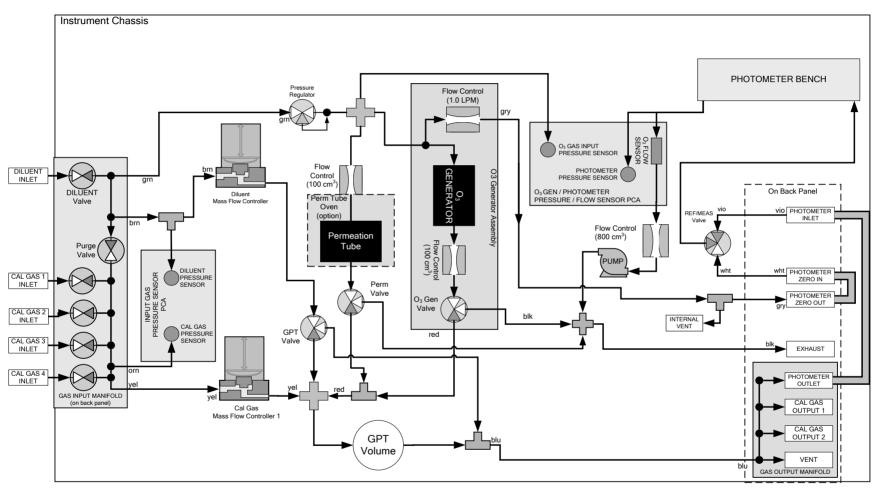
Figure 2-29. Pneumatic Flow with Permeation Generator
