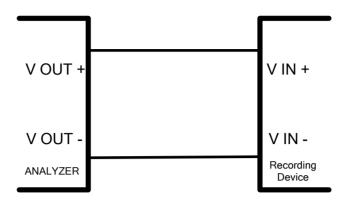
Figure 2-63. Setup for Calibrating the Analog Output Signals
