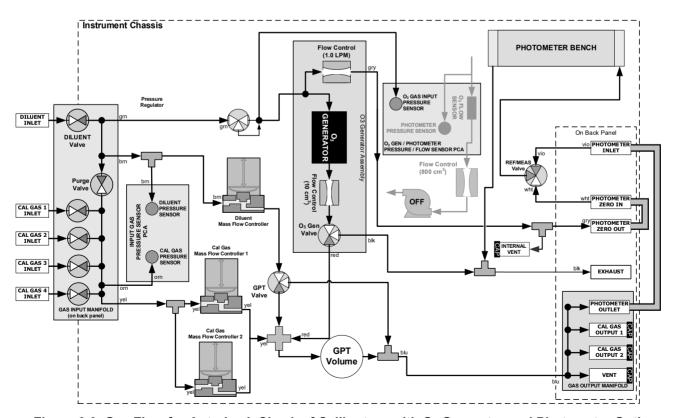
Figure 6-9. Gas Flow for Auto-Leak Check of Calibrators with O<sub>3</sub> Generator and Photometer Option
