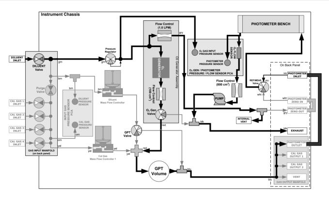
Figure 8-17. O<sub>3</sub> Photometer Gas Flow – Measure Cycle
