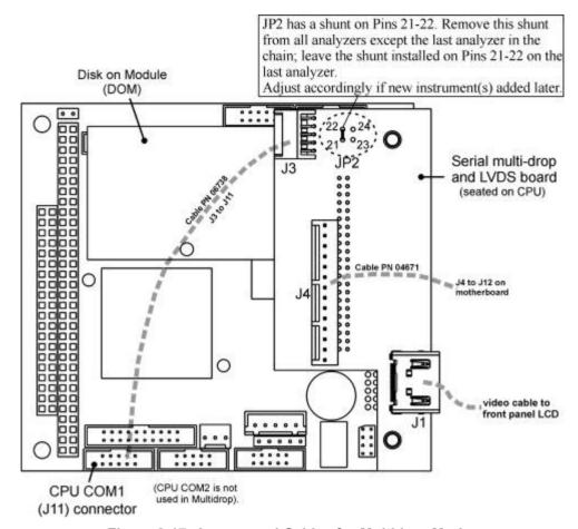
Figure 2-17. Jumper and Cables for Multidrop Mode
