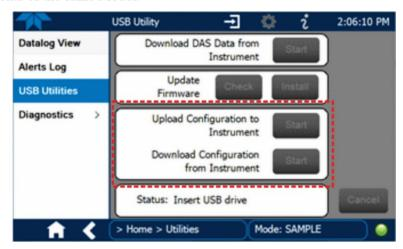
Figure 2-65. Configuration Transfer
