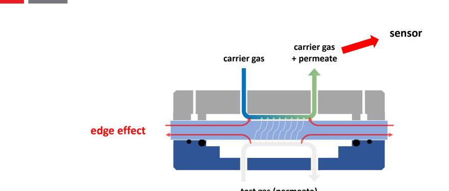
test gas (permeate) e.g. oxygen, carbon dioxide or humidified nitrogen
