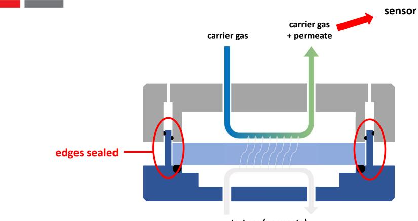
test gas (permeate) e.g. oxygen, carbon dioxide or humidified nitrogen
