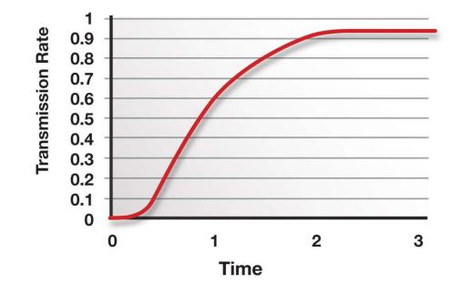
Measurement is finished when the permeate flow through the sample comes to an equilibrium
