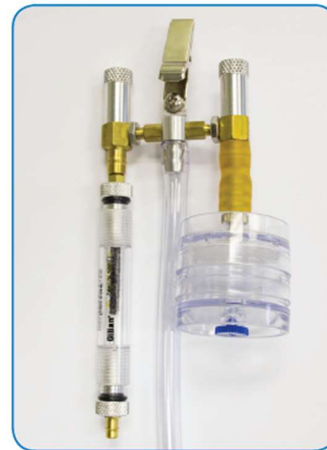
Bottom Access Model Shown with Sorbent Tube Holder and Filter Cassette
