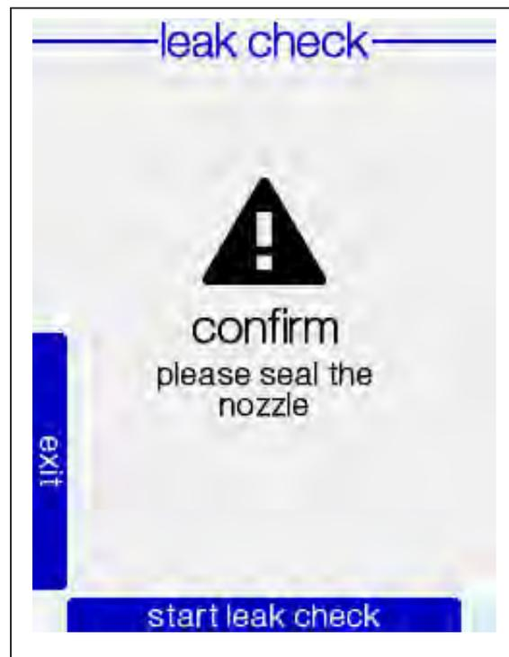
Assemble the sampling line as specified by the the adopted sampling standard and close inlet of the nozzle then press **START**.
