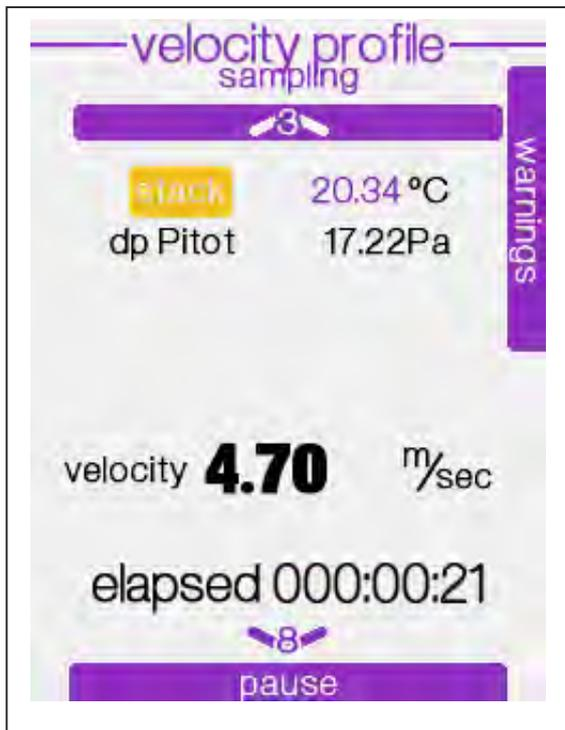
On the screen the velocity value will be displayed and the measure will start. The measure will go on until the time set is reached or user stops it.
