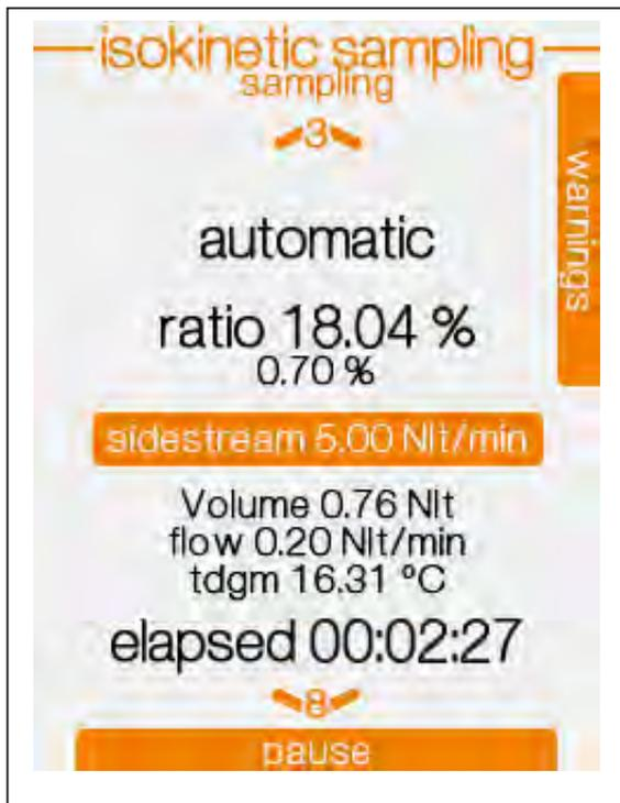
Before starting sampling process, set the sidestream nominal flow that the ADS must follows.
