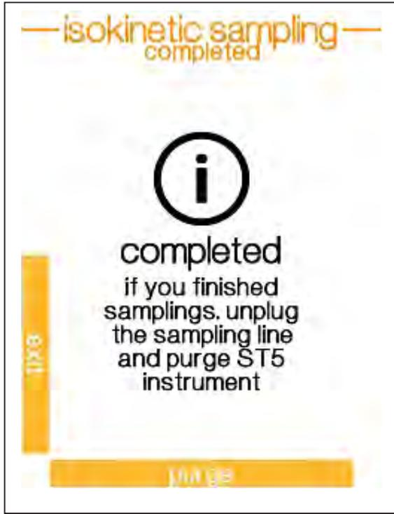
At the end of the sampling a pump purge is suggested in order to clean the pump
