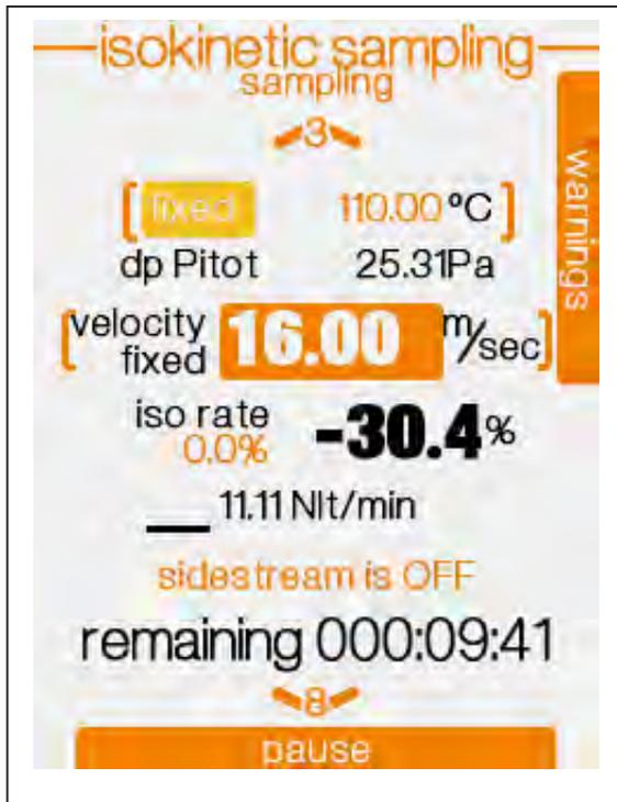
Velocity value will be displayed between parenthesis and the indication [ velocity fixed ] will appear
