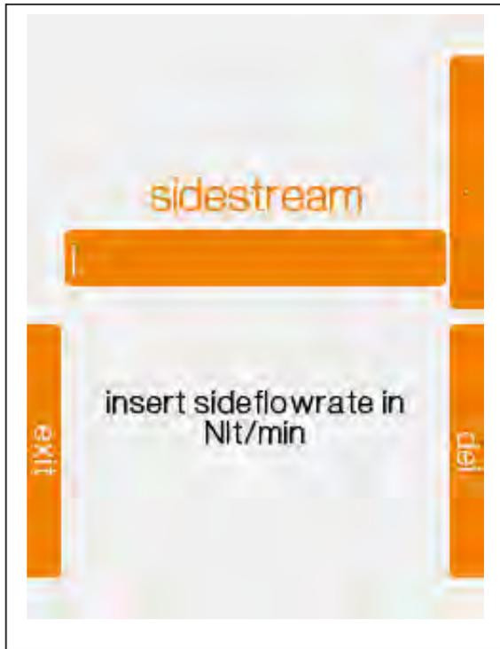
Set the sidestream flow setpoint selecting “side-stream 5.00 Nlt/min” and pressing ENTER key.
