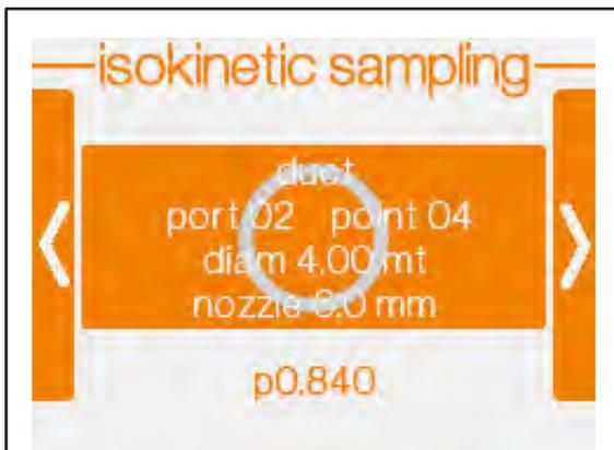
The main screen shows the actual duct specifications, to enter a new duct or edit an existing one, press **ENTER**. Press the **OPTION** and select.
