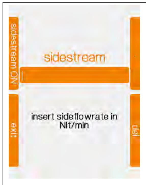
Enter the flowrate value set for the side sampling pump as Nl/min.
