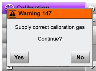
...make sure that the needle is exposed to the appropriate calibration gas, and then tap **Yes**.
