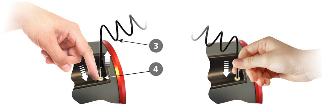
1. Push downwards on the sleeve ④ to release the hose ③, then pull the hose upwards and out of the connector.
