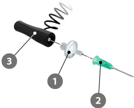
During use of the device, dust will over time be sucked through the measuring gas system, and therefore the filter **1** will have to be replaced regularly.
