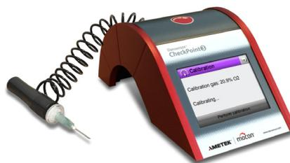
...place needle on the table next to the device to make sure that it measures the surrounding O<sub>2</sub> content, then tap **Yes**.
