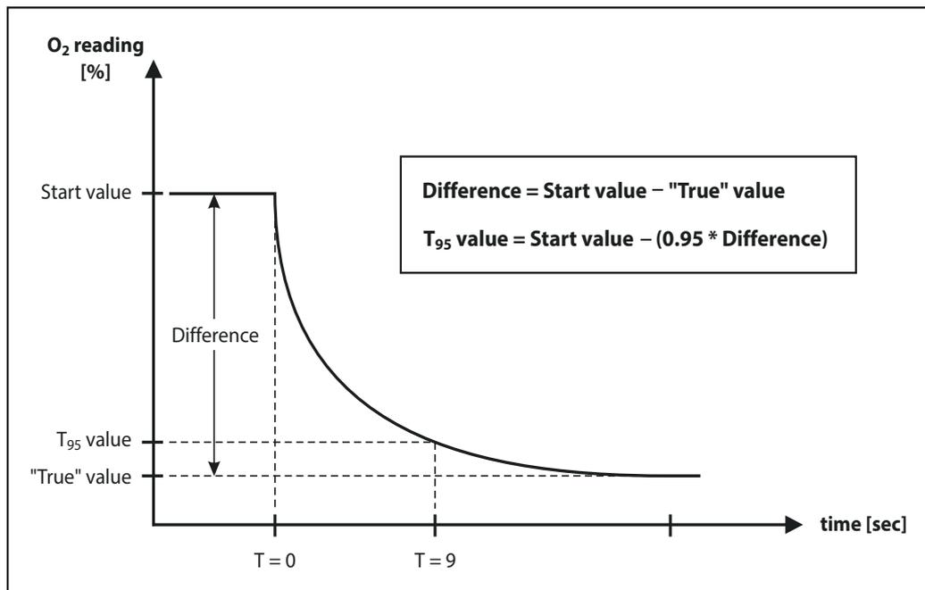
Consequently this means that if there is a large difference in the O<sub>2</sub> concentrations between two consecutive measurements, 2 or 3 measurements must be performed to obtain a more accurate result.
