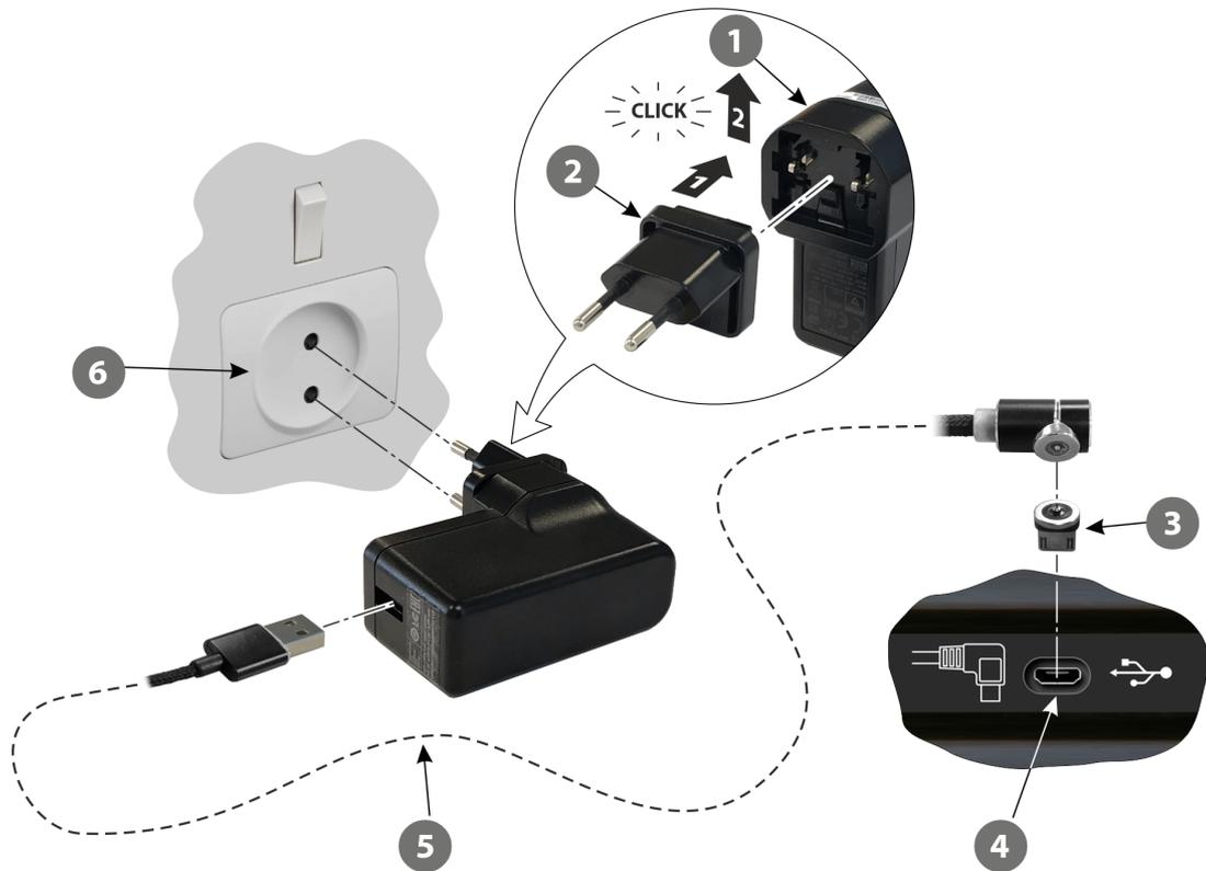
1. Assemble the power supply ① with the appropriate plug ② (see detail) - see [page 11](#) for plug compatibility details.
