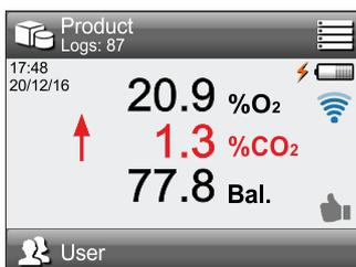
If any alarm limits have been defined, the results are shown in different colors - see *"The Measuring screen"* on page 18 for details.
