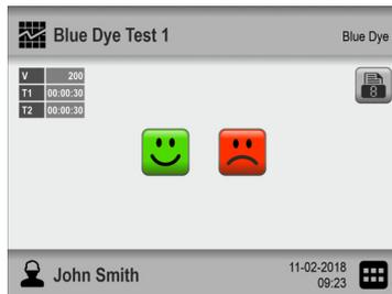
Thus, if you press the 😊 button, the test result will subsequently be indicated and registered as **OK**, whereas pressing the 😞 button will indicate and register the result as **Error**.
