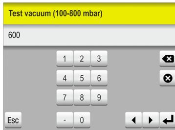
...then enter the required test vacuum (ex. 600 mbar) and press
