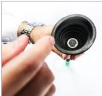
**Tighten the filter with your fingers and, if necessary, use the 13mm socket for final tightening.**
