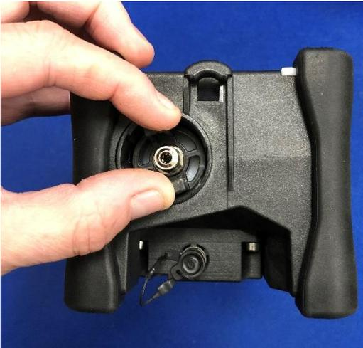
Unlock the filter by turning it counterclockwise and remove it.
