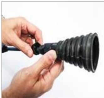
**Replace and hand-tighten the rubber housing.**
