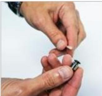
**Remove the old tubing from the quick-connect fitting.**
