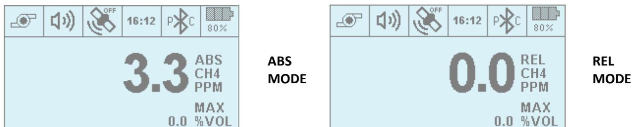
Note: The choice of absolute or relative mode is stored as non-volatile configuration. Each time the instrument is turned on, it will start using the same measurement mode it was using previously.
