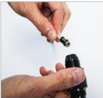
**Hold the tube, unscrew the filter holder, and remove the quick-connect fitting from inside the filter holder.**
