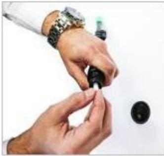
**Replace the discarded filter with a new cellulose filter.**
