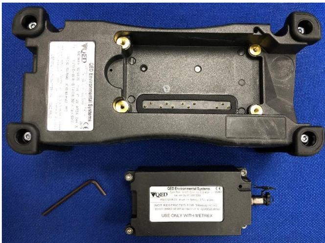
The picture shows the battery removed from the instrument
