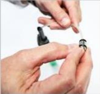
**Connect the replacement tubing to the quick-connect fitting.**
