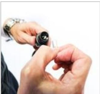
**Remove the cellulose dust filter from the end of the filter holder.**
