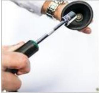
**Using a 13mm socket, unscrew the bronze dust filter and remove it from its position inside the rubber housing**
