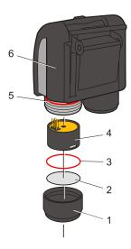
Before lamp cleaning or replacement, the the MiniPID Sensor must be removed.
