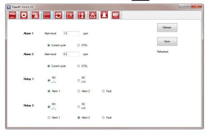
You can set each alarm to operate when the STEL or Current level of Benzene reaches a set value in ppm.
