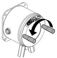
Turn counter-clockwise to unscrew the front cover.
