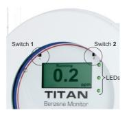
LEDs Green Titan is operating correctly.
