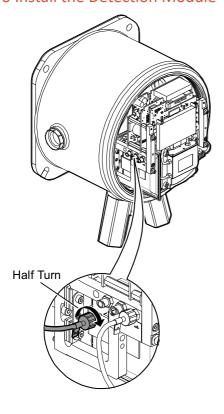
Check the identification of the pneumatic tubes and connectors.
