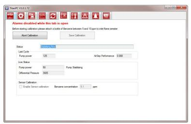
Attach a bottle of between 5 and 10ppm Benzene to the inlet flame-arrestor before you start calibration. This ensures the benzene is flowing through the Titan system before the start of the calibration.
