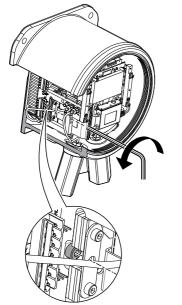
Two holes in the front of the Detection Module give access to the screws.
