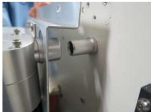
Figure 2-7 Dilution Flow System SCC Alignment
