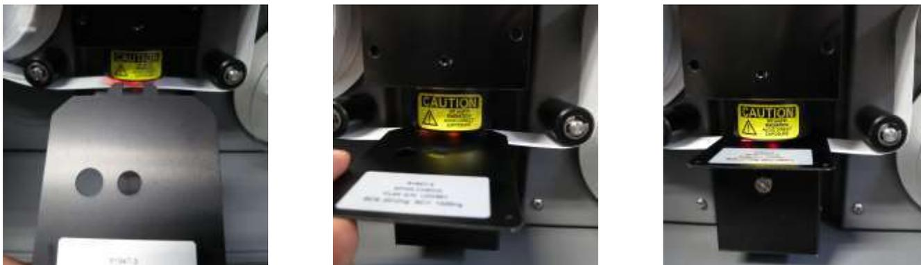
Figure 5-14 Inserting the Neutral Density Span Membrane
