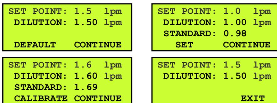
Figure 5-6 The BC 1054 Dilution Flow Calibration Screens
