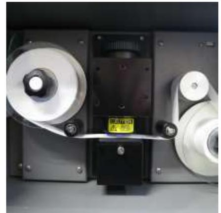
**Figure 5-10 Removing the Measurement Head Cover**
