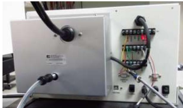
**Figure 2-10 Dilution Flow System Installed**
