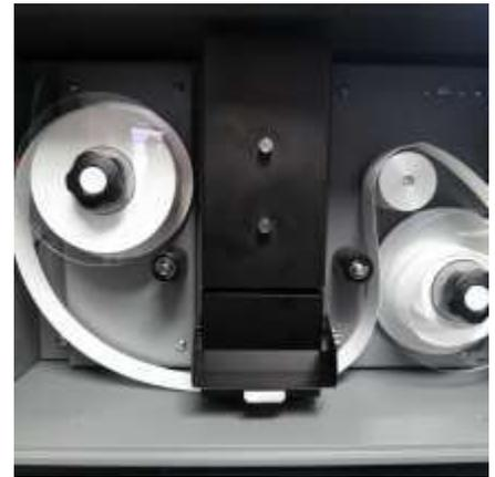
**Figure 5-9 Loosening the Tape for Cover Removal**
