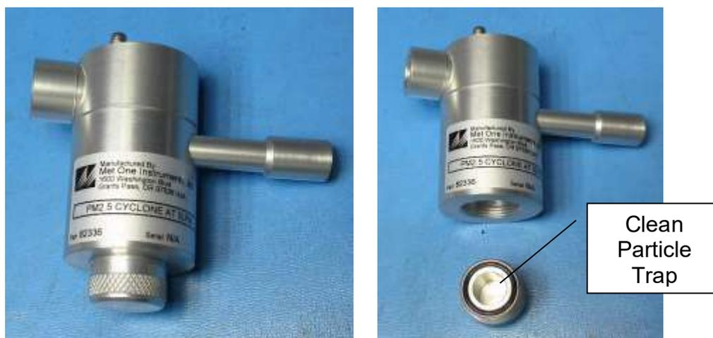
Figure 6-4 Unscrew and clean particle trap
