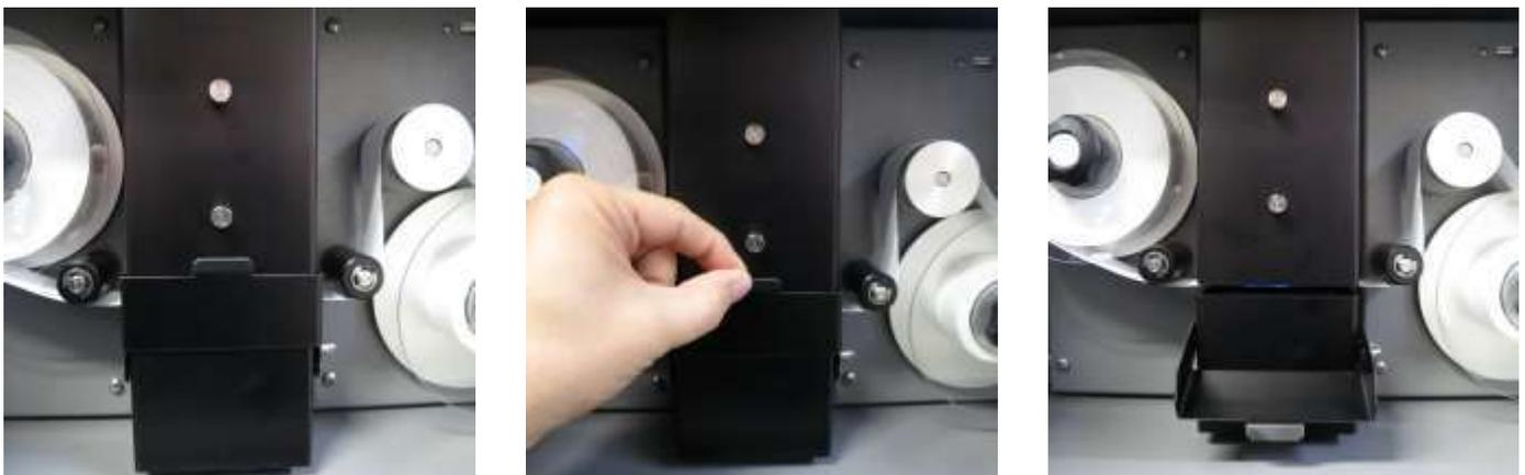
Figure 5-8 Opening the Tape Slot Access Door
