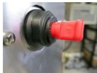
Figure 6-1 Leak Check Sealing Plug Installation
