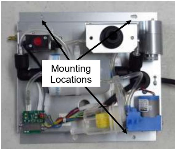
**Figure 2-8 Dilution Flow System Mounting Screw Locations**
