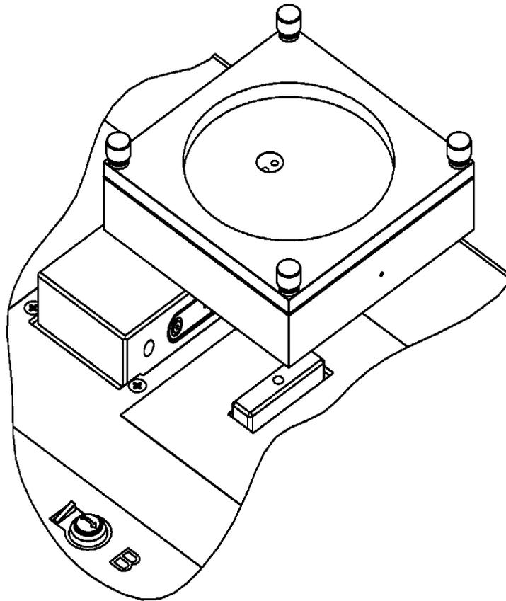
**Figure 3-3: Installing a Test Cartridge**
