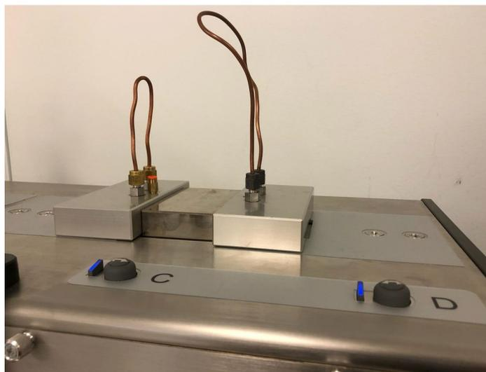
**Figure 3-1: Individual Zero with a Loop**
