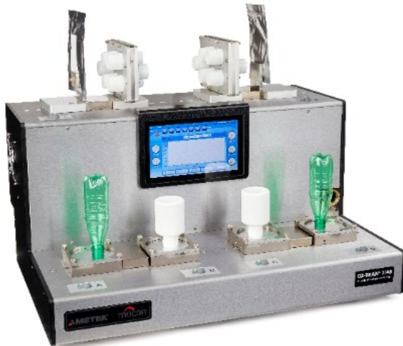
Figure 5-1: Packages are testing on OX-TRAN MODEL 2/48
