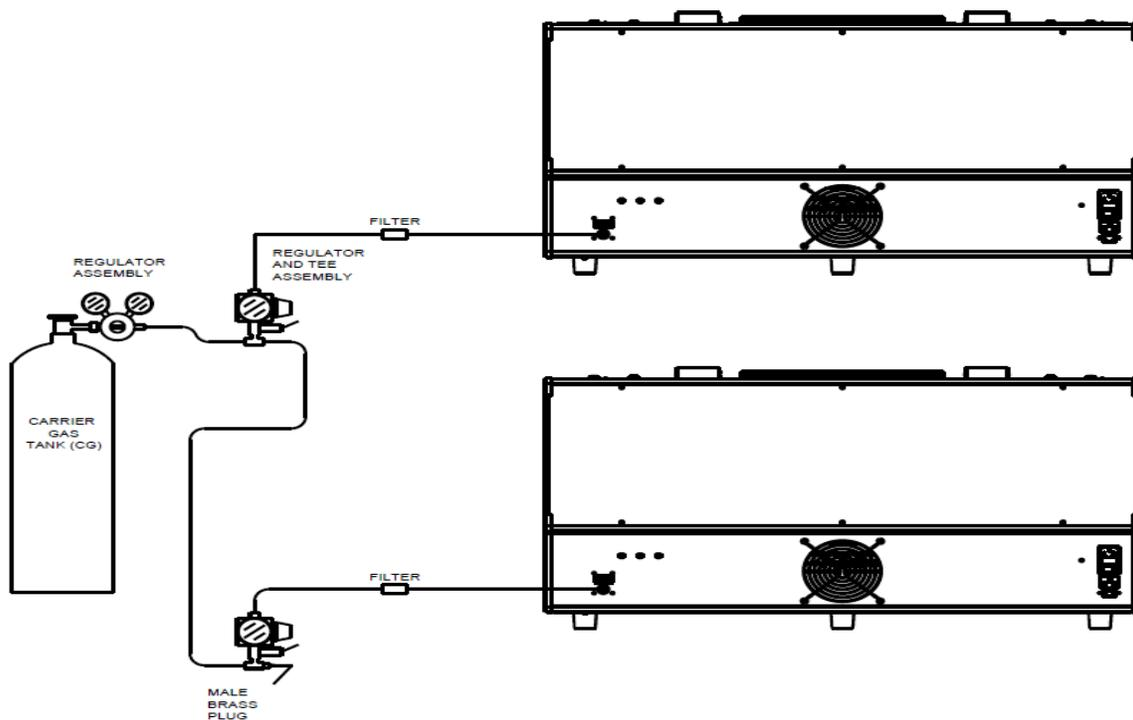
**Figure 2-6: System Plumbing Connection Diagram**
