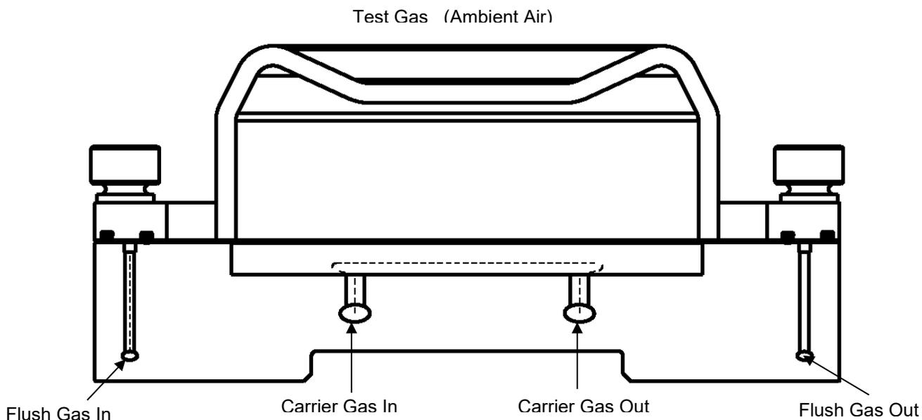
Figure 1-2: An OX-TRAN Model 2/48 Permeation Cell
