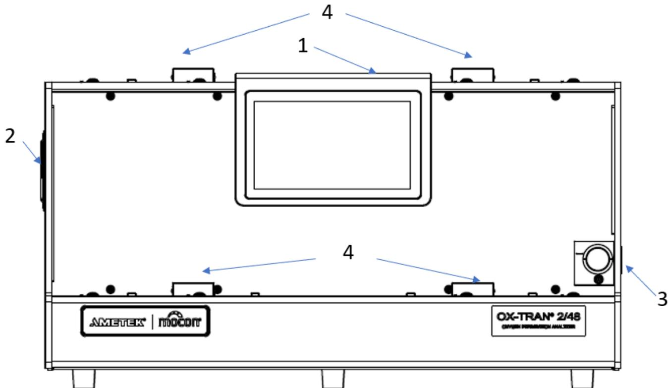
**Figure 2-1: Front Panel Parts and Controls**
