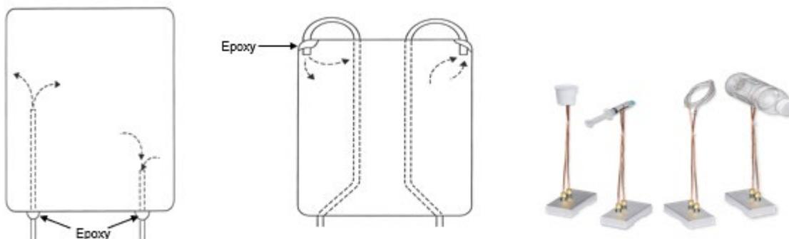
**Figure 5-4: Tube Mounted Packages**
