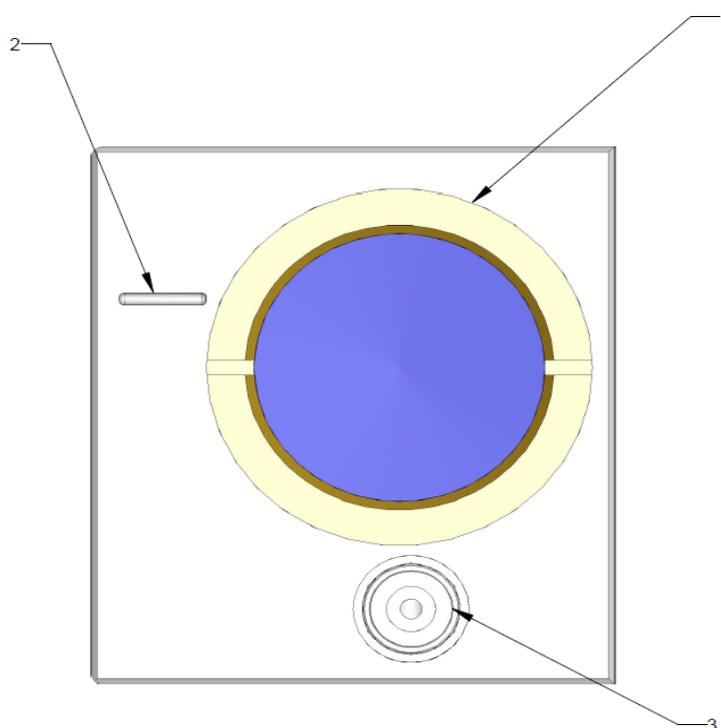
**Figure 3-2: Humidifier Fill Port and Controls**
