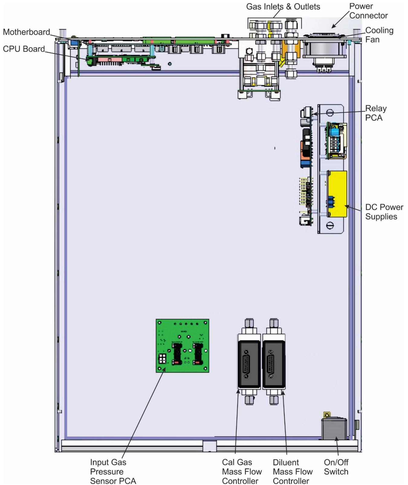
**Figure 2-3. Calibrator Internal Layout – Top View – Base Unit**
