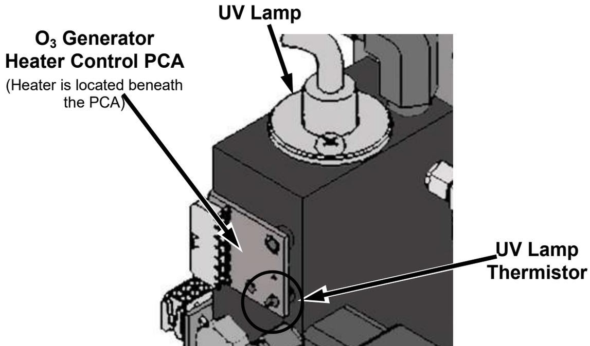
Figure 8-16. O<sub>3</sub> Generator Temperature Thermistor and DC Heater Locations
