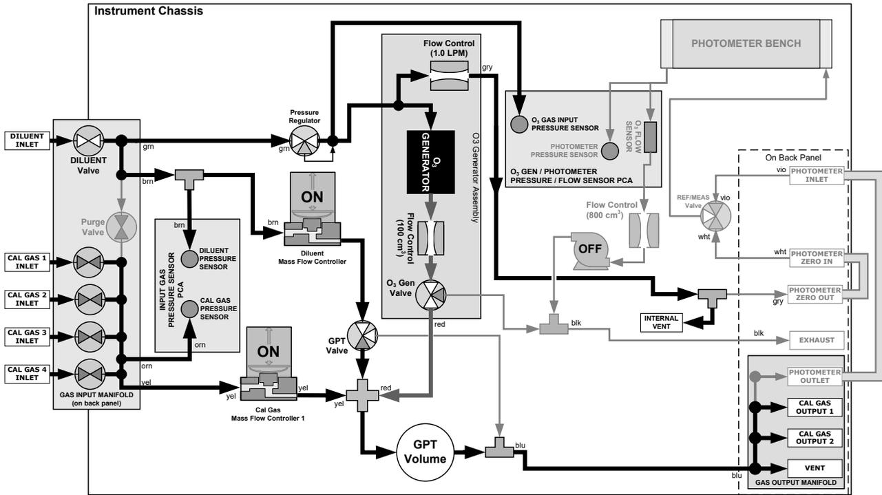
Figure 3-12. Gas Flow with O<sub>3</sub> Options during GPT Mode
