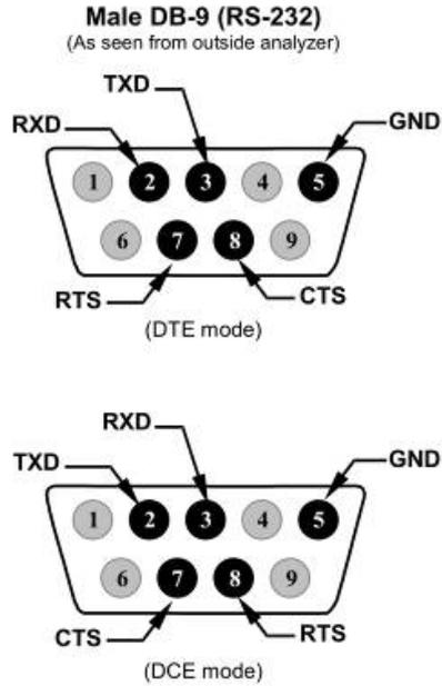
**Figure 2-15. Rear Panel Connector Pin-Outs for RS-232 Mode**
