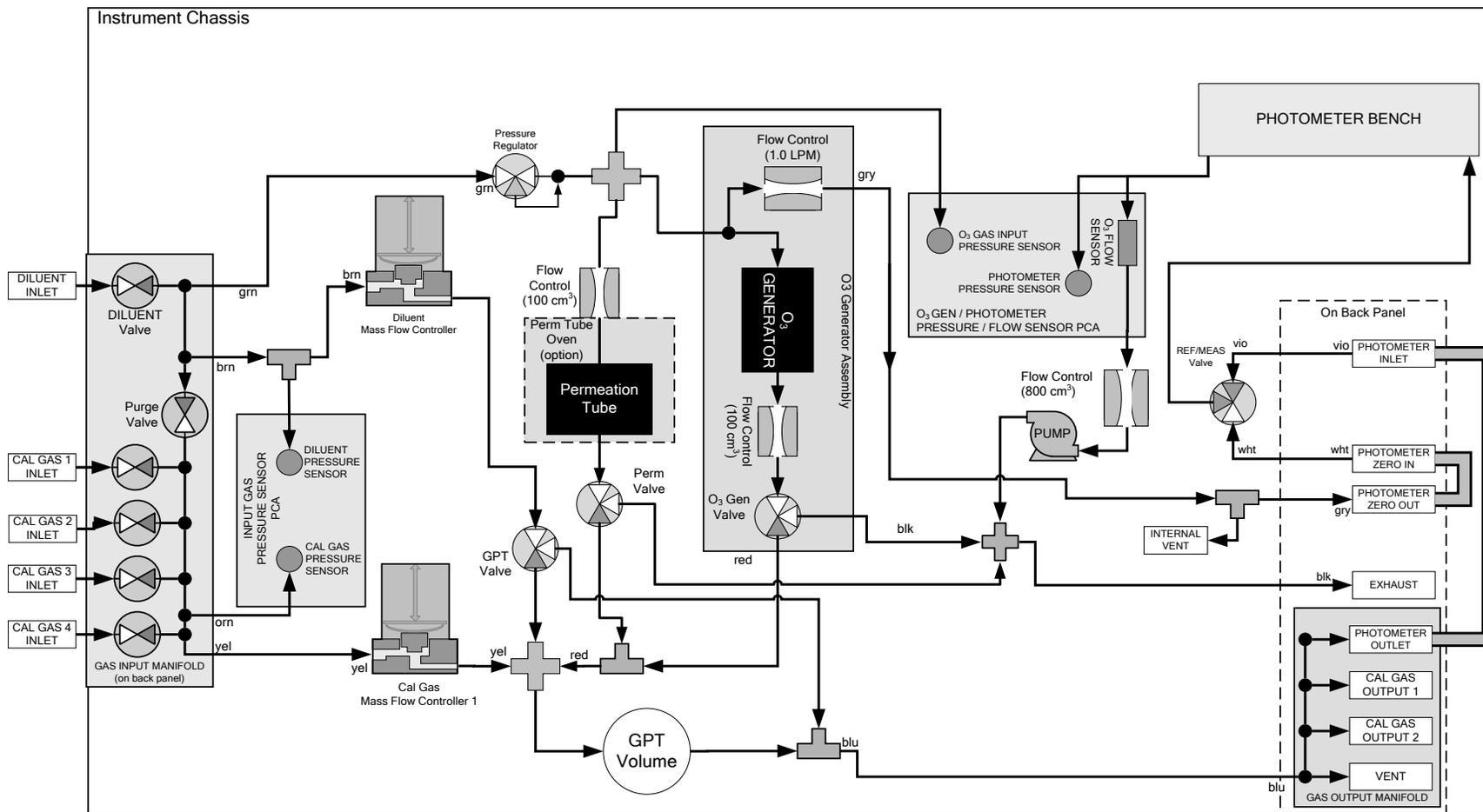
Figure 2-29. Pneumatic Flow with Permeation Generator
