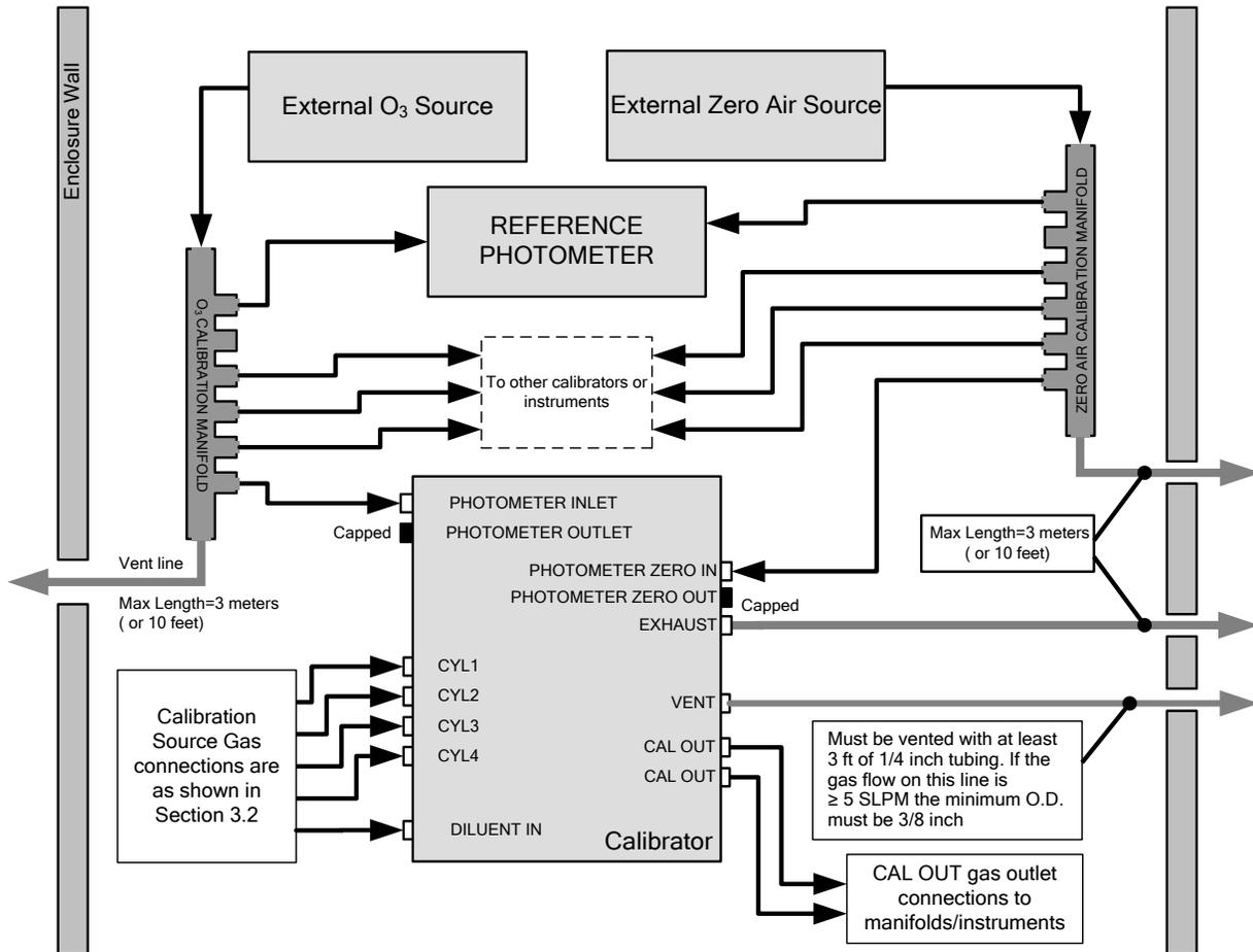
**Figure 5-7. External Photometer Validation Setup with Calibration Manifolds**
