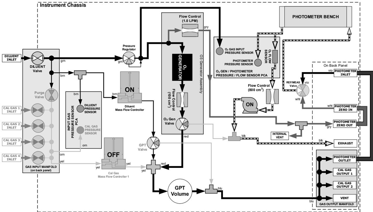
Figure 3-4. Gas Flow with O<sub>3</sub> Options when Generating O<sub>3</sub>
