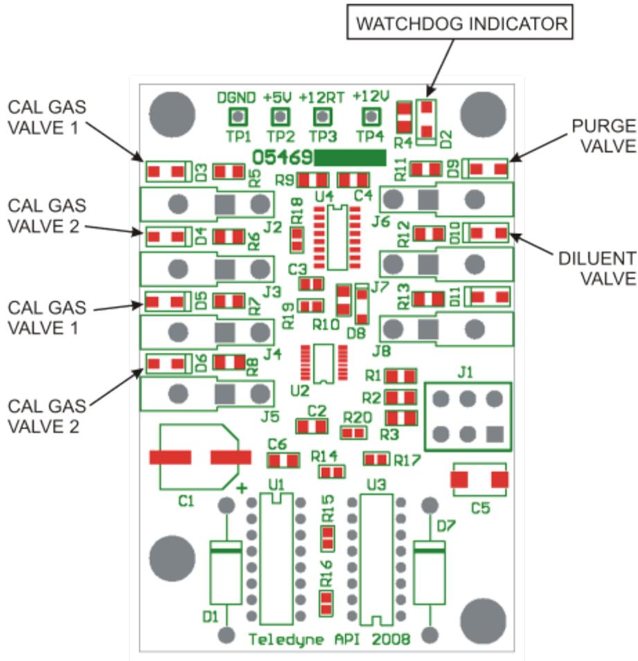
Figure 8-8. Status LED Locations – Valve Driver PCA
