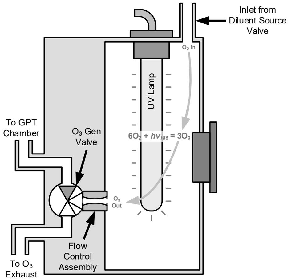
Figure 8-12. O<sub>3</sub> Generator Internal Pneumatics
