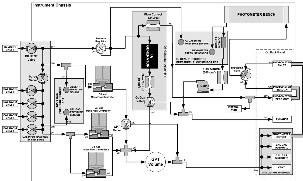
Figure 2-27. Calibrator with Multiple Calibration Gas MFCs and O<sub>3</sub> Options 1A and 2A Installed
