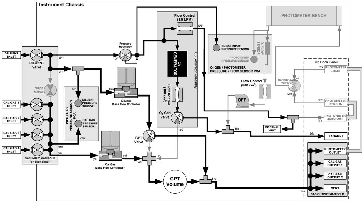
Figure 3-3. Gas Flow with O<sub>3</sub> Options when Generating Non-O<sub>3</sub> Source Gas
