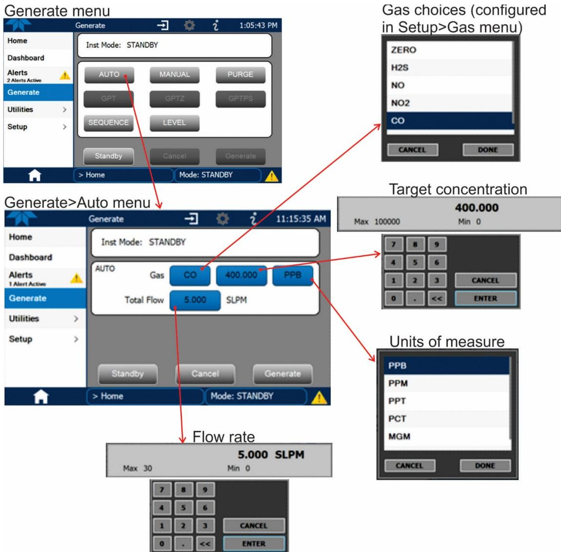
Figure 3-6. Auto Generate Calibration Mixtures
