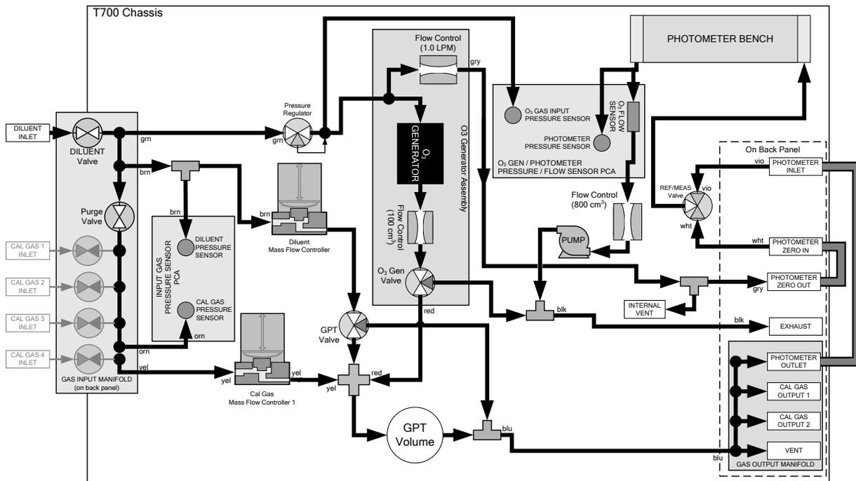
Figure 3-9. Gas Flow with O<sub>3</sub> Options during Purge mode
