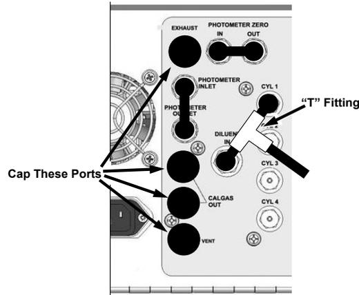
**Figure 6-7. Gas Port Setup for Auto-Leak Check Procedure**
