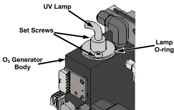
**Figure 6-11. O<sub>3</sub> Generator UV Lamp Location**
