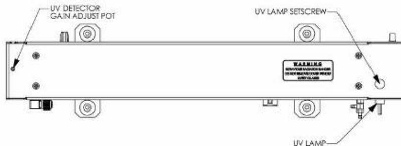
**Figure 6-10. Photometer Assembly – Lamp Adjustment / Installation**
