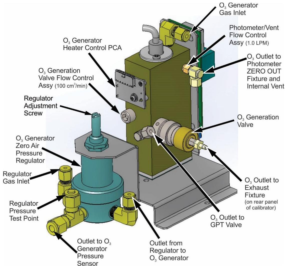
**Figure 8-13. O<sub>3</sub> Generator Valve and Gas Fixture Locations**
