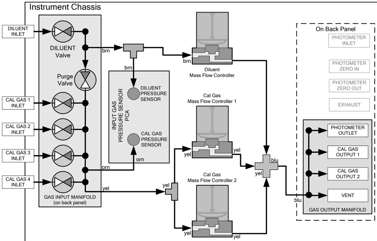
Figure 2-26. Basic Calibrator with Multiple Calibration Gas MFCs
