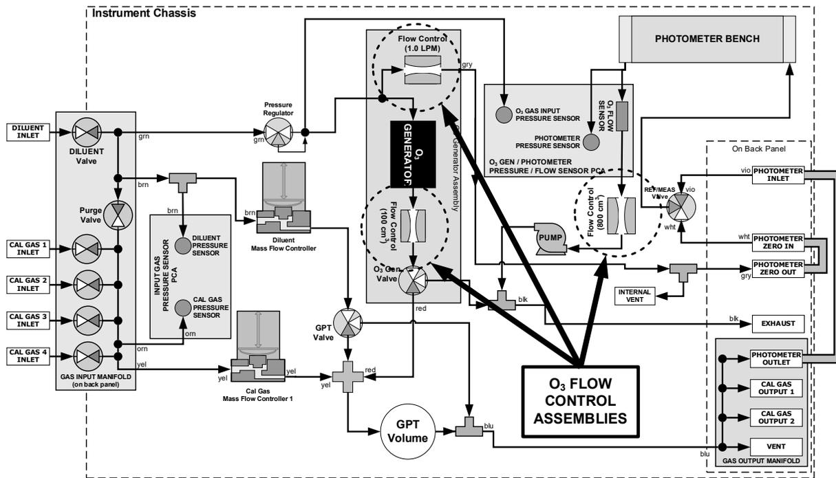
**Figure 8-1. Location of Gas Flow Control Assemblies with O<sub>3</sub> Generator Installed**
