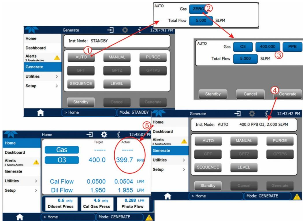
Figure 5-5. O<sub>3</sub> Photometer Performance Verification
