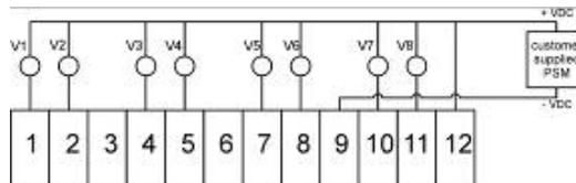
**Figure 2-13. Options 48C & 48D Connections, Customer-supplied PSM to Pin 12 (+) & Pin 9 (-)**
