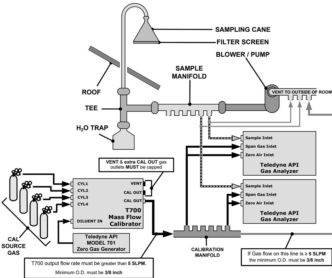
**Figure 2-21. Setup – Connecting the Calibrator to a Calibration Manifold**
