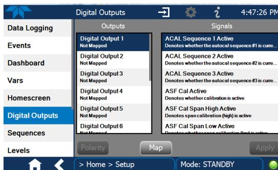
Figure 2-57. Digital Outputs Setup
