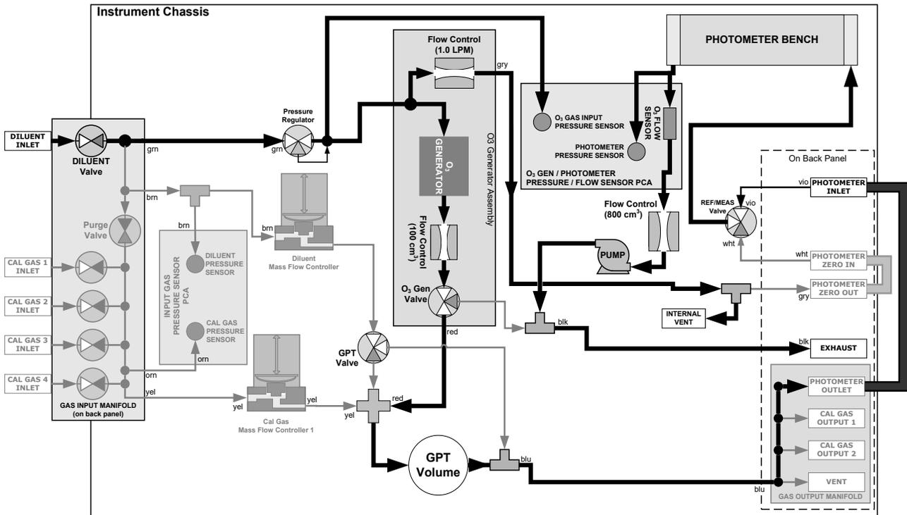
**Figure 8-17. O<sub>3</sub> Photometer Gas Flow – Measure Cycle**
