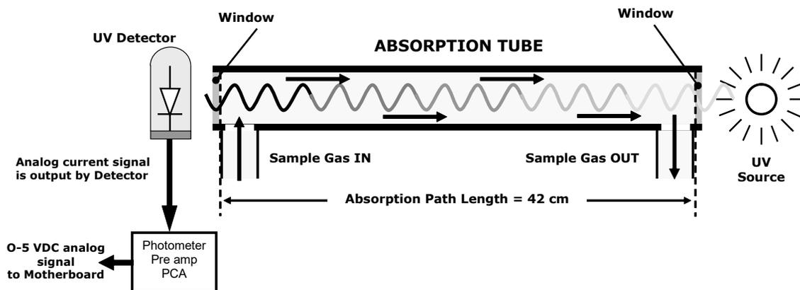
Figure 8-19. O<sub>3</sub> Photometer Absorption Path
