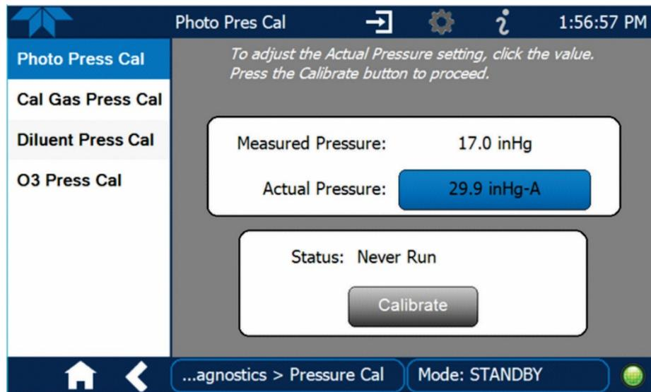
Figure 5-14. O3 Photometer Pressure Sensor Calibration Page
