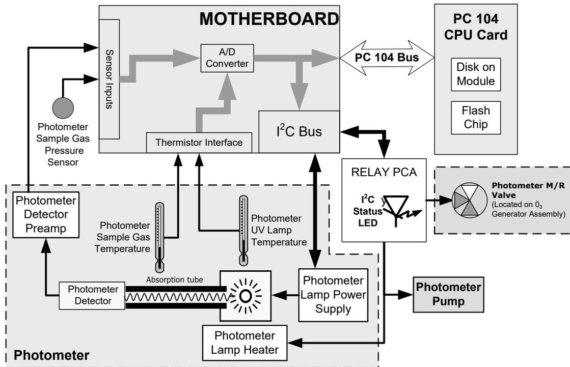
**Figure 8-21. O<sub>3</sub> Photometer Electronic Block Diagram**
