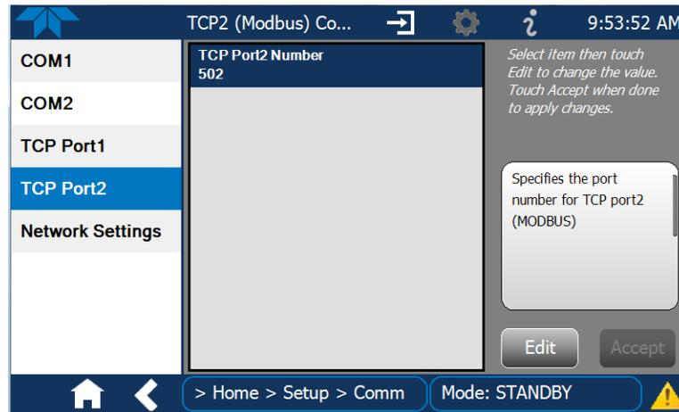
Figure 4-1. MODBUS via Ethernet
