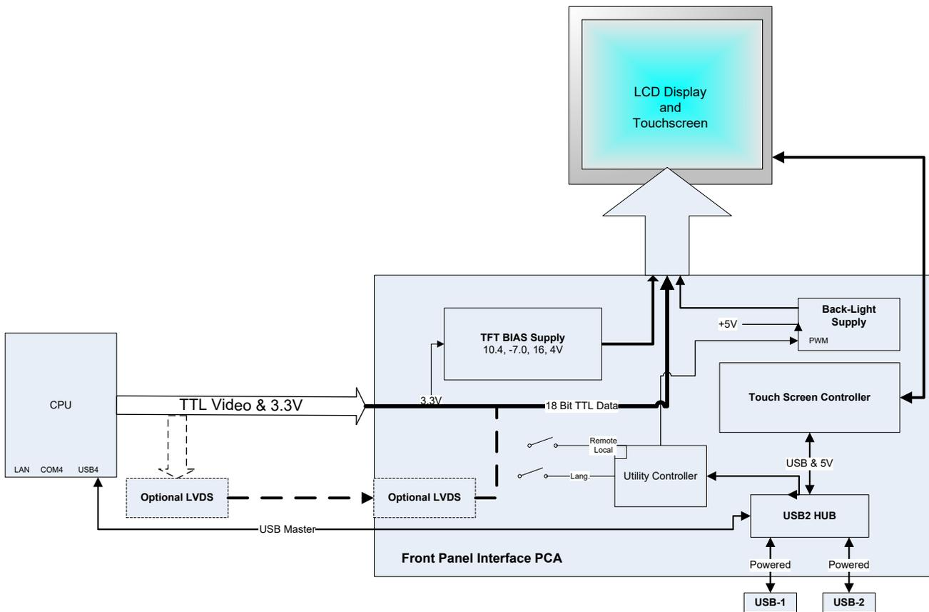
**Figure 8-10. Front Panel Display Interface Block Diagram**
