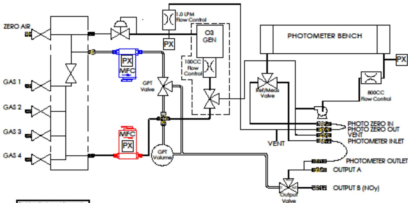
Figure 2-31. Internal Pneumatics with Optional Dual Gas Output (NO<sub>y</sub> – Special)
