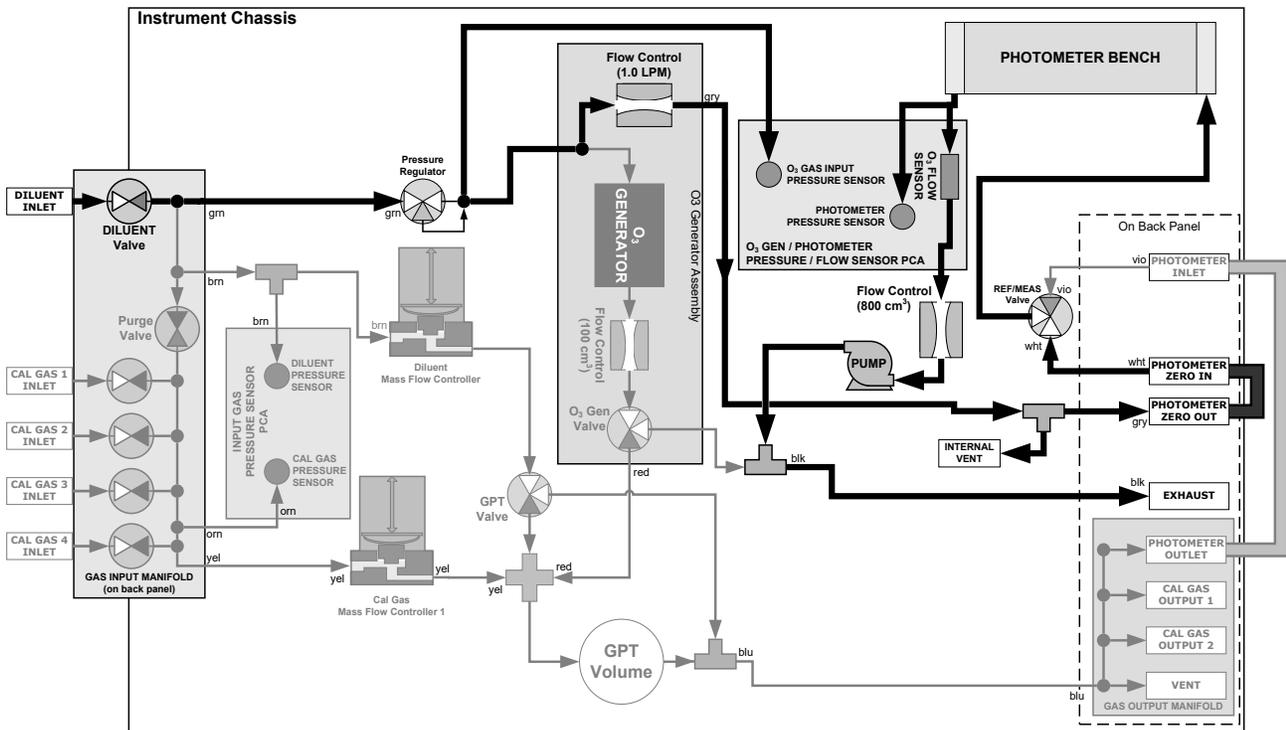
**Figure 8-18. O<sub>3</sub> Photometer Gas Flow – Reference Cycle**
