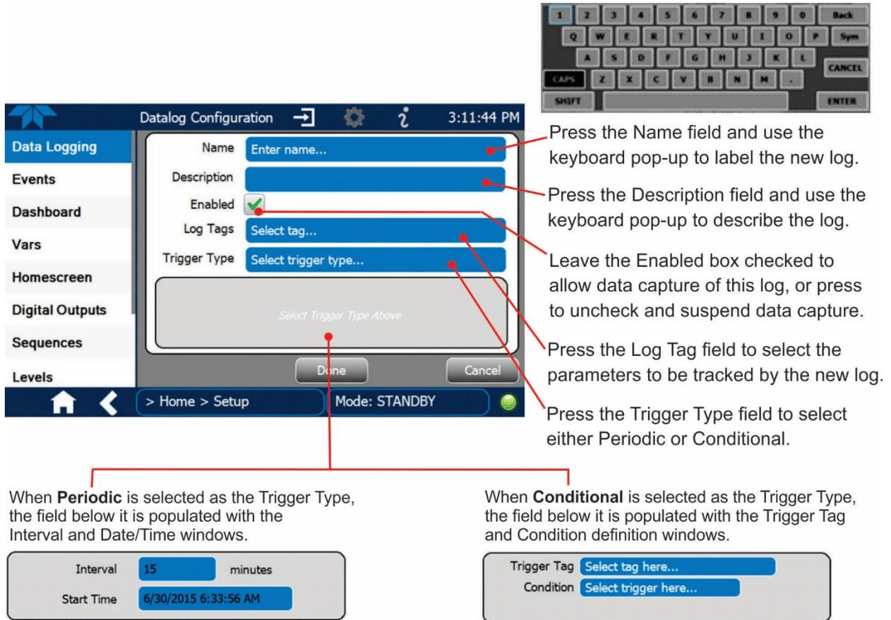
The screenshot shows the 'Datalog Configuration' screen. The left sidebar contains menu items: Data Logging, Events, Dashboard, Vars, Homescreen, Digital Outputs, Sequences, and Levels. The main area has fields for Name, Description, Enabled (checked), Log Tags, and Trigger Type. Below these is a large grey area with the text 'Select Trigger Type Above'. At the bottom are 'Done' and 'Cancel' buttons. A keyboard pop-up is shown in the top right corner.
