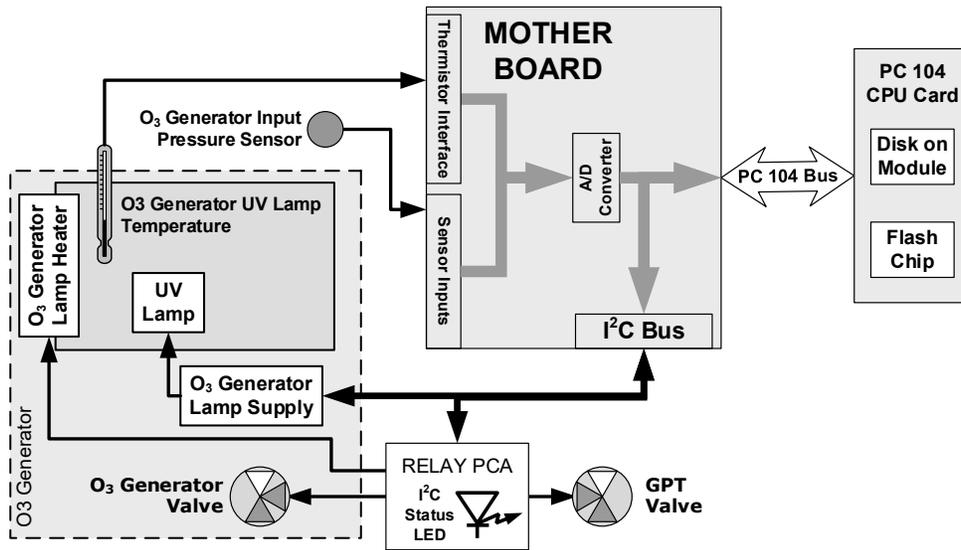
Figure 8-14. O<sub>3</sub> Generator – Electronic Block Diagram
