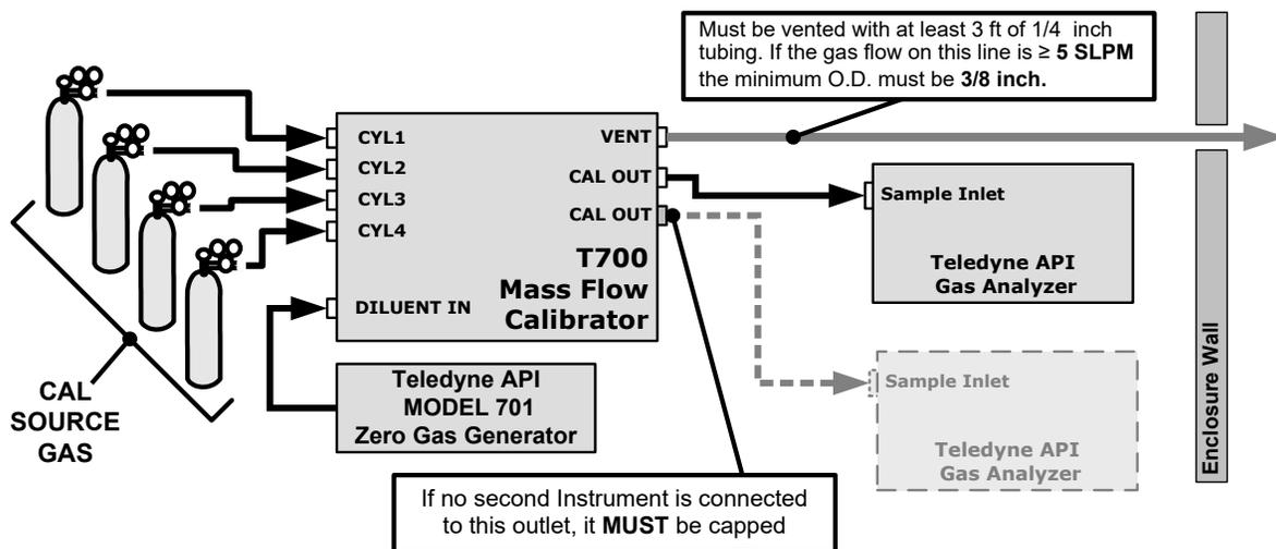
**Figure 2-19. Setup – Connecting the Basic Calibrator to a Sample Manifold**
