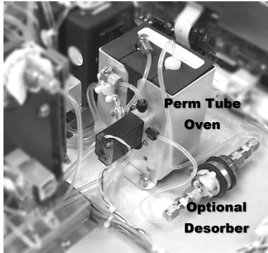
Figure 2-28. Permeation Tube Gas Generator Option
