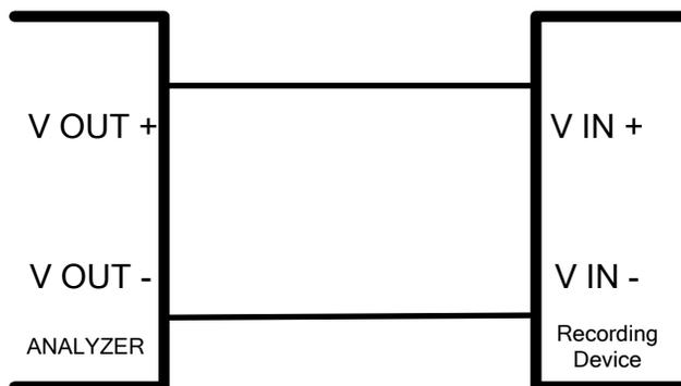
**Figure 2-63. Setup for Calibrating the Analog Output Signals**
