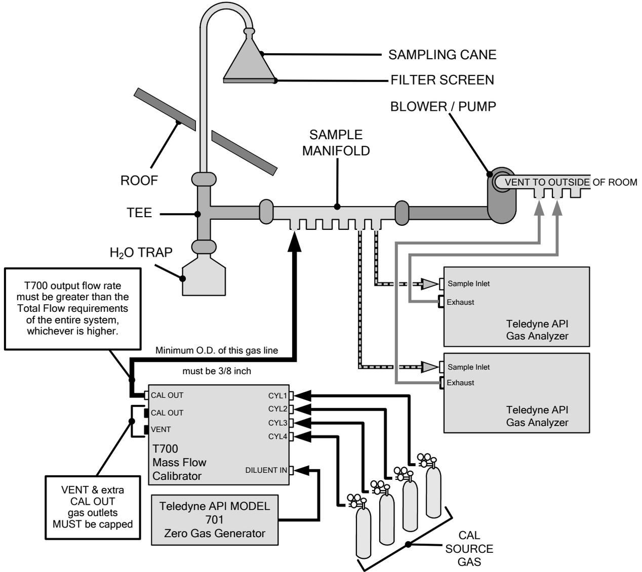
**Figure 2-20. Setup – Connecting the Calibrator to a Sample Manifold**
