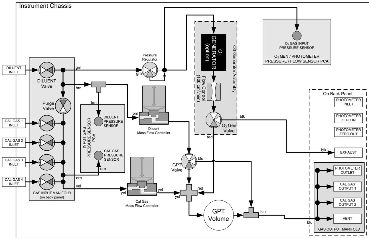
Figure 2-24. Internal Pneumatics for Calibrator with Optional O<sub>3</sub> Generator and GPT Chamber
