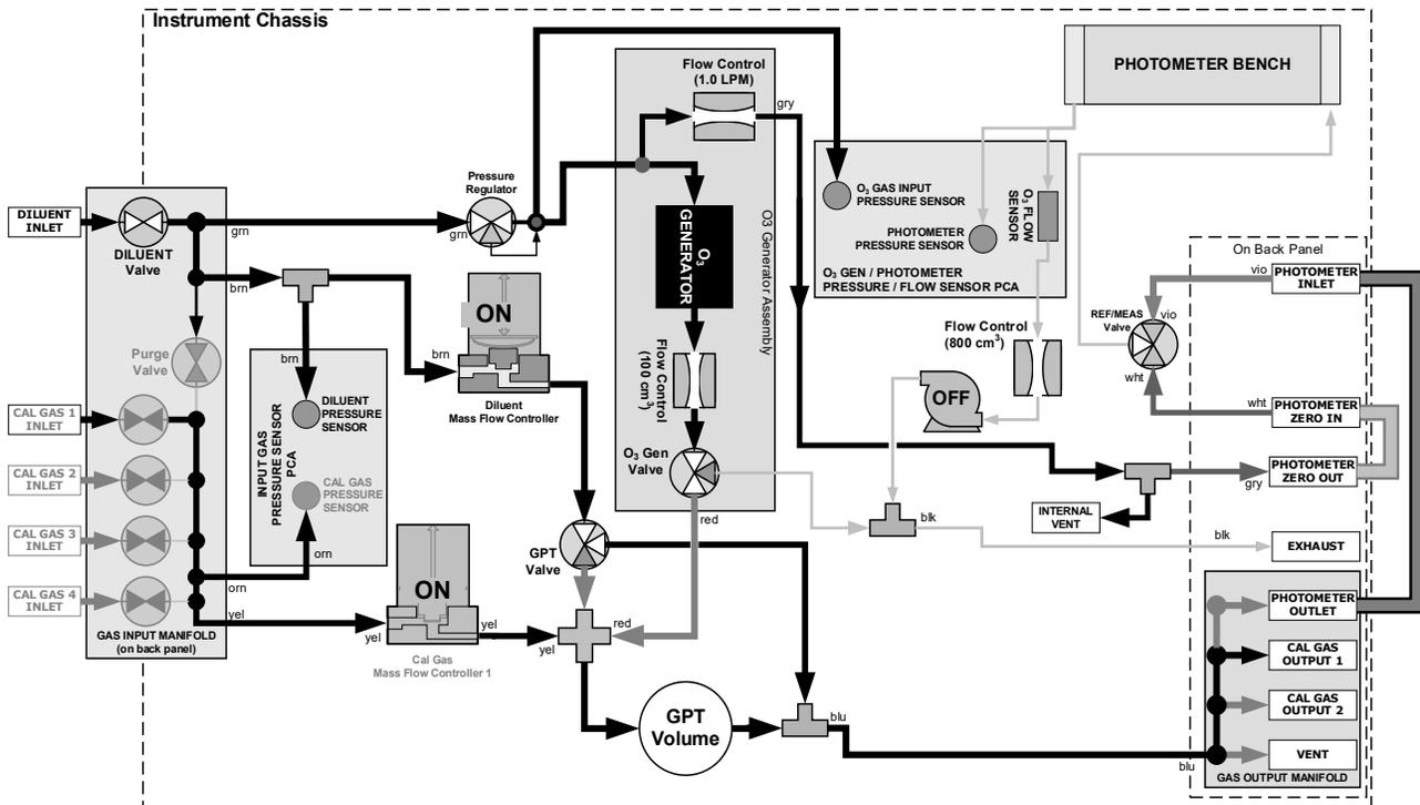
Figure 3-10. Gas Flow with O<sub>3</sub> Options during GPTZ Mode
