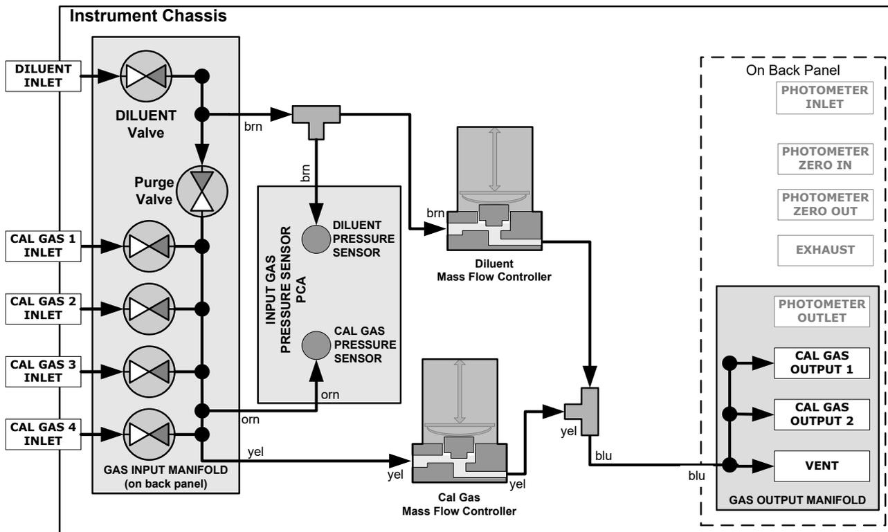
**Figure 2-23. Calibrator Pneumatic Diagram – Base Unit**
