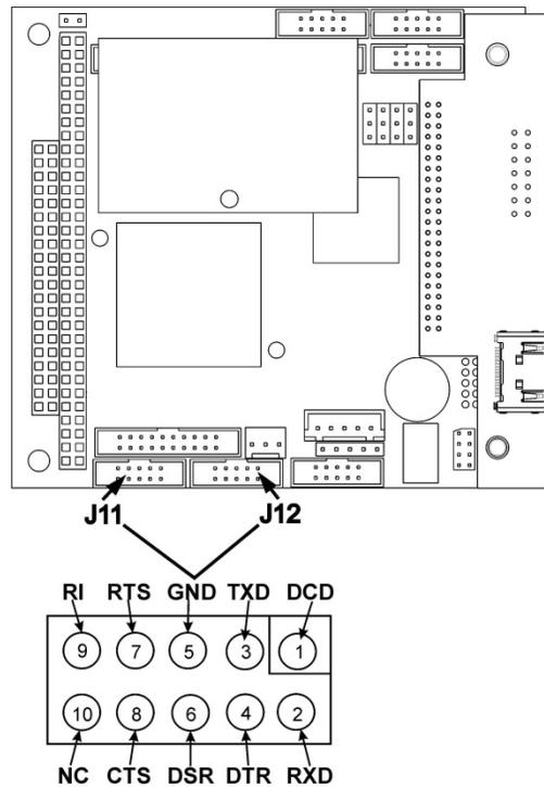
**Figure 2-16. Default Pin Assignments for CPU COMM Port Connector (RS-232).**
