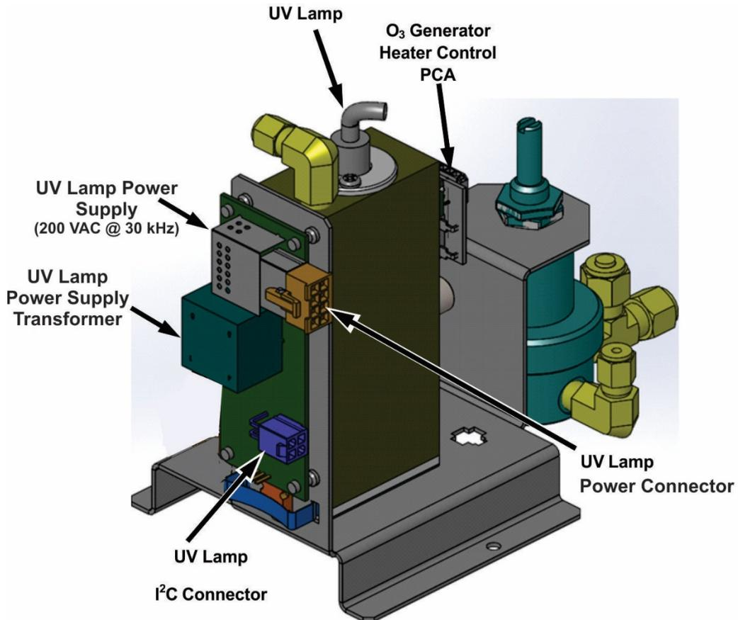
Figure 8-15. O<sub>3</sub> Generator Electronic Components Location
