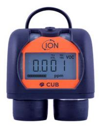
Cub is the world's smallest, lightest personal PID monitor for the accurate detection of volatile organic and total aromatic compounds. With market leading parts-per-billion (ppb) sensitivity, Cub gives an early warning of hazardous gases, including benzene, before they reach levels which are harmful.
