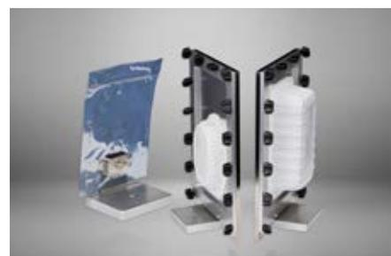
*The Package Adapter Cartridge is designed for testing complete containers including closures and seals allowing you to verify that your entire package meets your permeation performance goals.*
