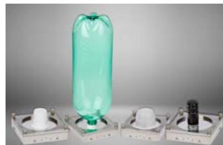
*No more messy sample prep! Using our disposable foils, just epoxy your sample to the foil, put it on the cartridge, tighten the 4 fasteners and you are ready to go. When testing is complete just dispose of the foil. No more scraping & cleaning to reuse.*
