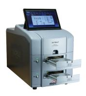
Interchangeable cartridge options such as package adapter, edge effect and reduced area cartridges expand testing capabilities
