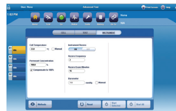
Digital testing include: Cell Temperature, Permeant Concentration, Instrument Rezero ON/OFF, Rezero Frequency
