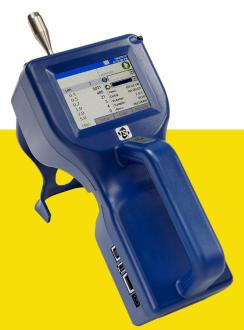
Multiple AeroTrak 9306 particle counter configurations can be conveniently stored and uploaded as needed using the TrakPro Lite Secure data download and reporting software supplied as standard.
