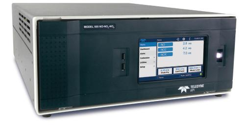
The Model 500 CAPS NO<sub>x</sub> analyzer uses superior Cavity Attenuated Phase Shift (CAPS) Spectroscopy to measure True NO<sub>2'</sub> NO<sub>x'</sub> and NO gases. The instrument combines direct NO<sub>2</sub> measurements with highly efficient gas phase titration (GPT) to convert and measure the NO gas component. An automatic baseline reference cycle accounts and compensates for any potential baseline drift due to varying environmental conditions.
