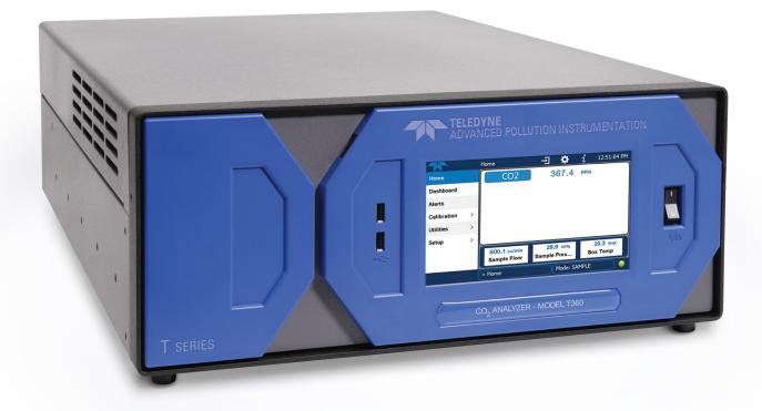
Using a gas filter correlation wheel, the Model T360  $CO_2$  analyzer measures carbon dioxide by comparing infrared energy absorbed by a sample to that absorbed by a reference gas according to the Beer-Lambert law.
